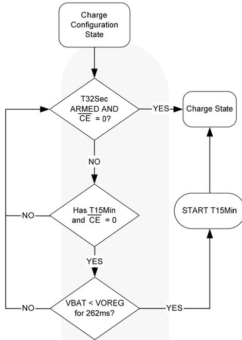
**Figure 39. Charge Configuration**
