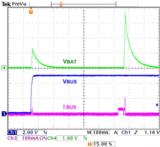
Figure 17. No Battery at  $V_{BUS}$  Power-up; FAN54010, FAN54013
