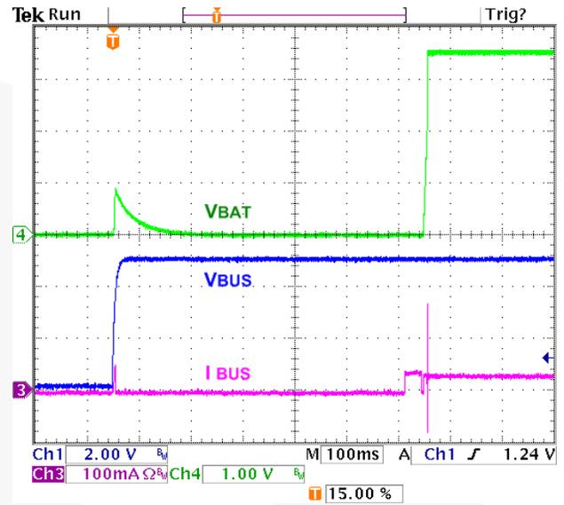
Figure 18. No Battery at  $V_{BUS}$  Power-up; FAN54012, FAN54015
