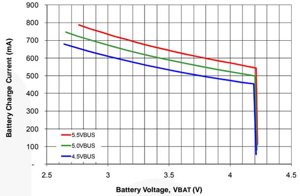
Figure 8. Battery Charge Current vs.  $V_{BUS}$  with  $I_{INLIM}=500mA$
