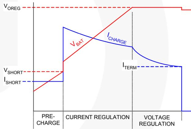
Figure 36. Charge Curve, I<sub>INLIM</sub> Limits I<sub>CHARGE</sub>
