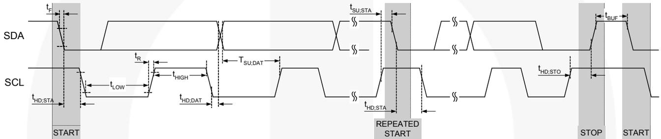
Figure 5. I<sup>2</sup>C Interface Timing for Fast and Slow Modes
