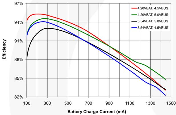
Figure 9. Charger Efficiency, No  $I_{INLIM}$ ,  $I_{CHARGE}=1,450mA$
