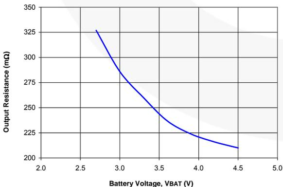
**Figure 43. Output Resistance (R<sub>OUT</sub>)**
