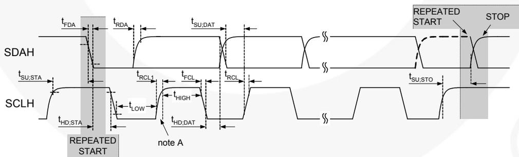
Figure 6. I<sup>2</sup>C Interface Timing for High-Speed Mode
