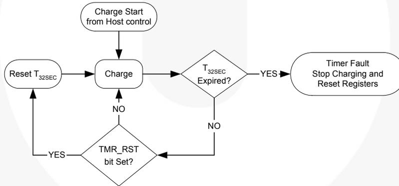
**Figure 42. Timer Flow Chart for FAN54011 and FAN54014**
