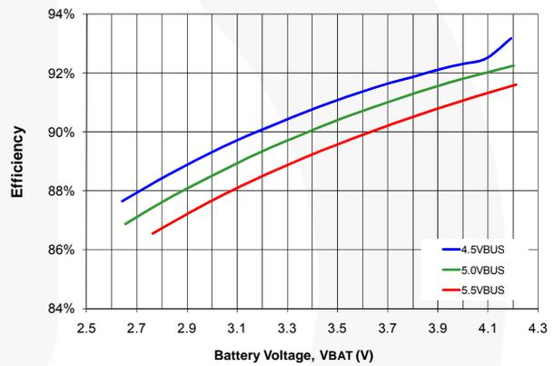
Figure 10. Charger Efficiency vs.  $V_{BUS}$ ,  $I_{INLIM}=500mA$
