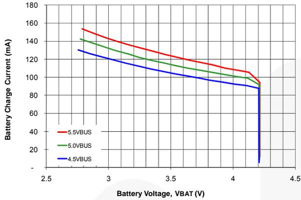
Figure 7. Battery Charge Current vs.  $V_{BUS}$  with  $I_{INLIM}=100mA$
