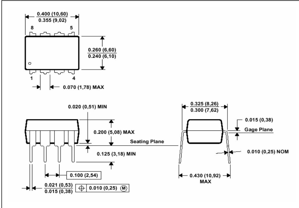
NOTE 1 : All linear dimensions are in inches ( millimeters ) .
