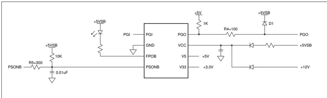
NOTE1 : The series resistor R5 at PSONB can not be omitted. ( R0 = 300Ω is suggested )
