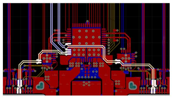
Figure 60. Complete USB2 Routing
