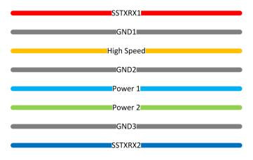
Figure 46. 8 Layer Board Stack Up
