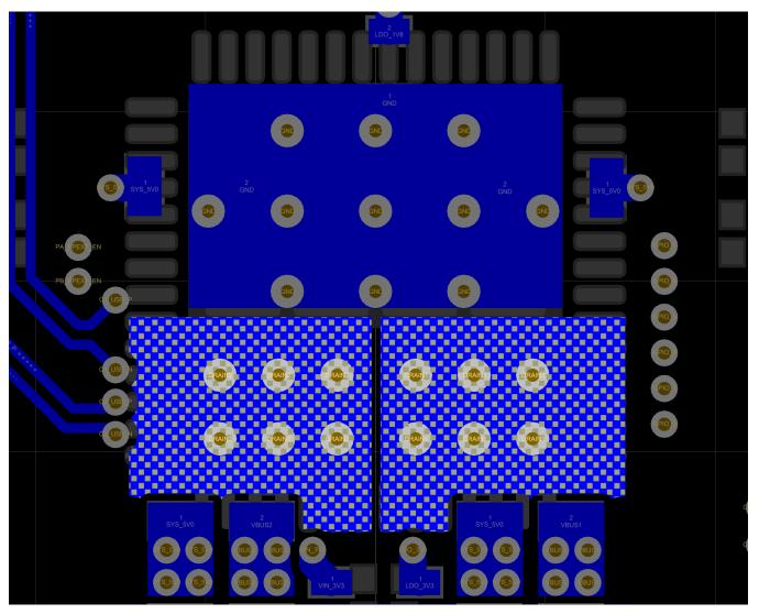
Figure 59. Figure 13. DRAIN1 and DRAIN2 Bottom Layer
