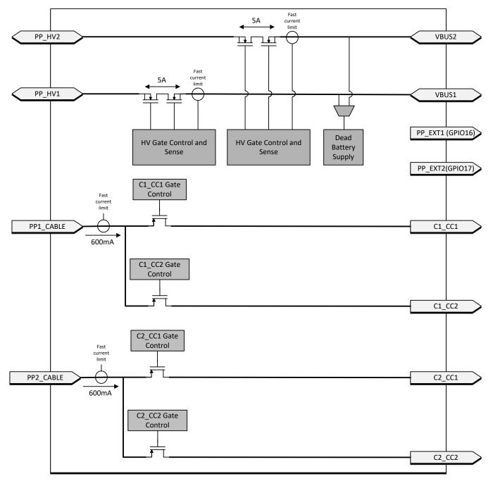
Figure 13. Port Power Switches
