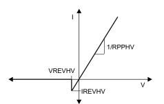
Figure 14. Comparator Mode (Source) Internal HV Switch I-V Curve
