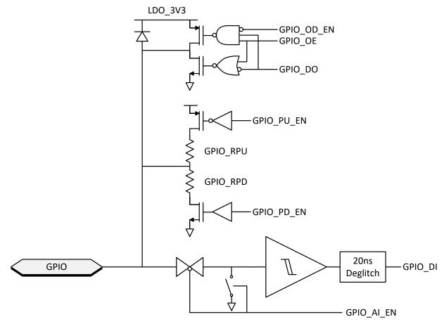
Figure 22. General GPIO Buffer
