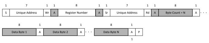
Figure 30. I<sup>2</sup>C Unique Address Read Register Protocol
