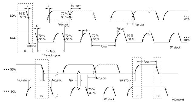
Figure 2. I<sup>2</sup>C Slave Interface Timing
