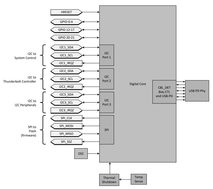
Figure 25. Digital Core Block Diagram
