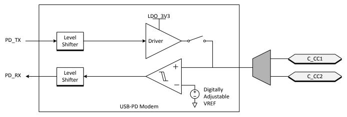
Figure 8. USB-PD BMC TX/Rx Block Diagram
