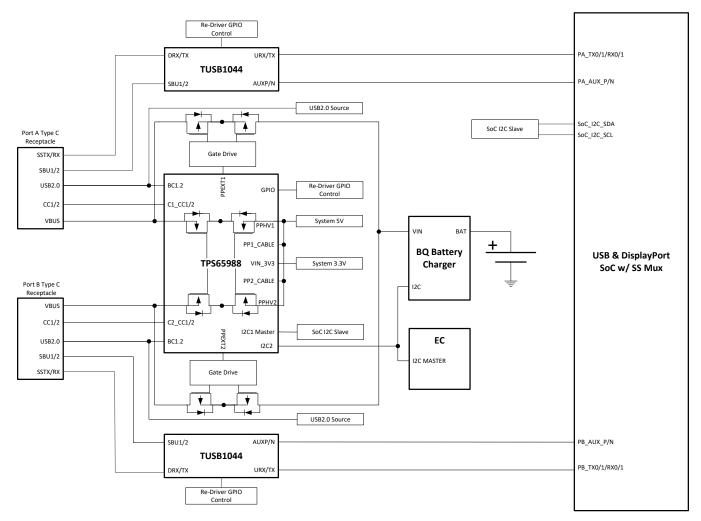
Figure 41. TPS65988 and SoC I2C w/ Re-Driver GPIO
