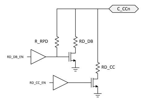
Figure 19. Dead Battery Pull-Down Resistor
