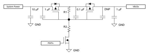
Figure 34. Simple Sink Power Path
