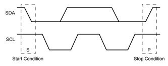
Figure 26. I<sup>2</sup>C Definition of Start and Stop Conditions
