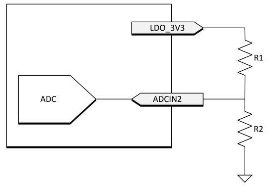
Figure 32. I<sup>2</sup>C Address Divider
