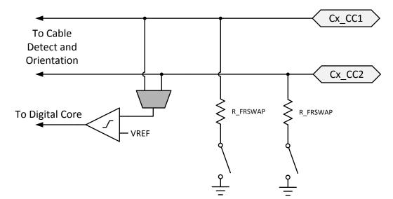
Figure 18. Fast Role Swap Detection and Signaling
