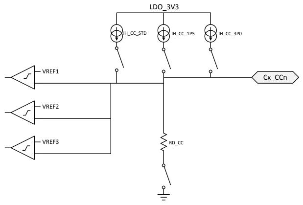
Figure 17. Plug and Orientation Detection Block
