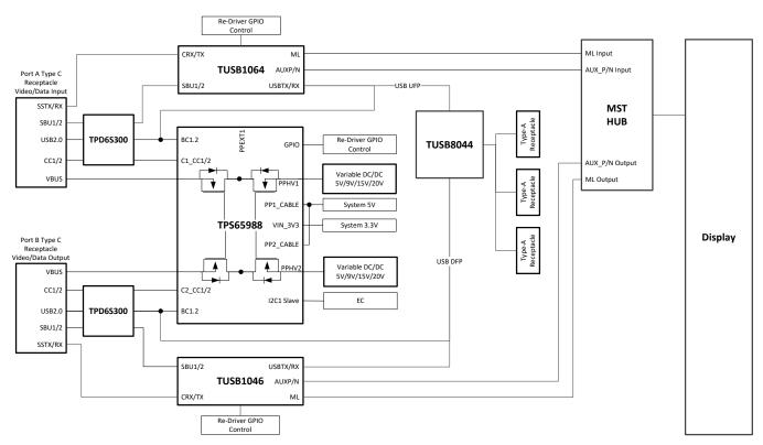
Figure 43. USB and DisplayPort Dock Block Diagram
