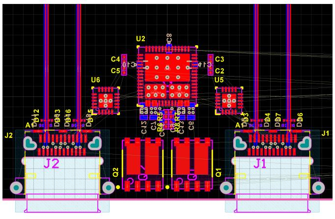
Figure 56. Protection Placement
