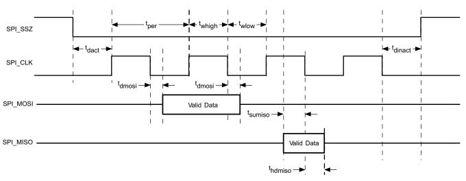
Figure 3. SPI Master Timing
