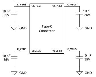
Figure 35. Type-C Connector VBUS Capacitors
