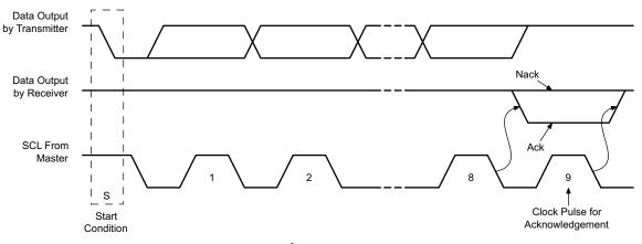
Figure 28. I<sup>2</sup>C Acknowledgment
