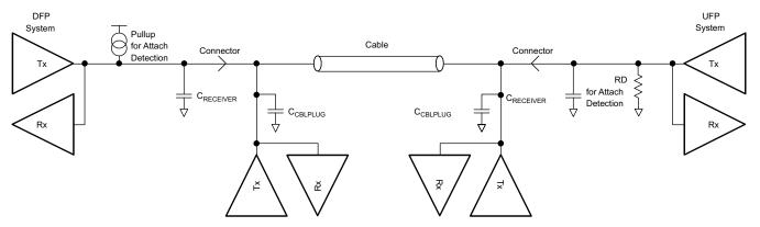
Figure 11. Example USB-PD Multi-Drop Configuration
