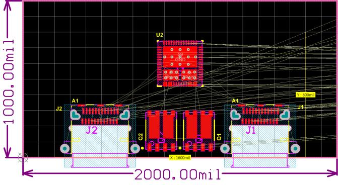
Figure 48. High Level Placement
