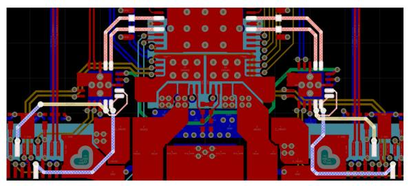
Figure 57. Complete CC Routing
