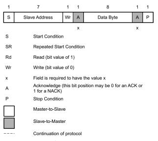
Figure 31. I<sup>2</sup>C Read/Write Protocol Key
