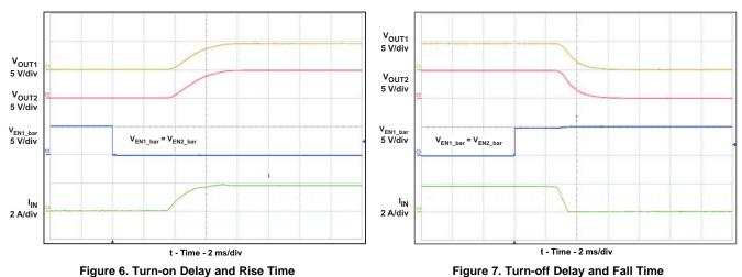
Figure 6. Turn-on Delay and Rise Time
