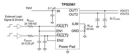
Figure 20. Auto-Retry Functionality With External EN Signal
