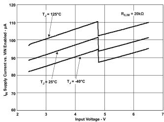
Figure 12.  $I_{IN}$  – Supply Current, Output Enabled –  $\mu A$
