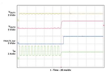
Figure 8. Full-Load to Short-Circuit Transient Response
