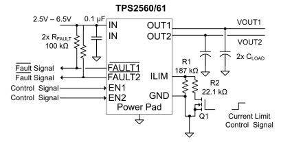
Figure 21. Two-Level Current-Limit Circuit
