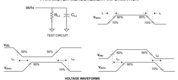
Figure 2. Test Circuit and Voltage Waveforms
