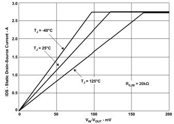
Figure 16. Switch Current Vs. Drain-Source Voltage Across Switch
