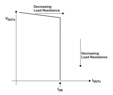
Figure 4. Output Voltage vs. Current-Limit Threshold
