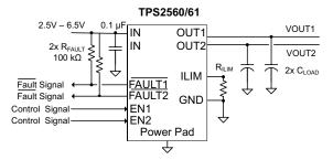
Figure 1. Typical Application as USB Power Switch
