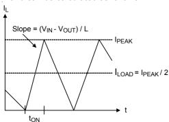
Figure 2. Boundary Condition of CCM/DEM
