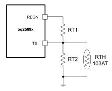
Figure 14. TS Resistor Network
