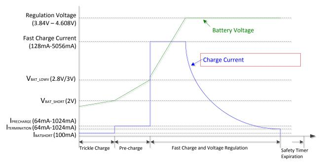
Figure 13. Battery Charging Profile
