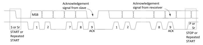
Figure 19. Data Transfer on the I<sup>2</sup>C Bus
