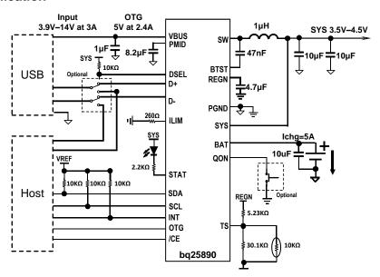
Figure 47. bq25890 with D+/D- Interface and USB On-The-Go (OTG)
