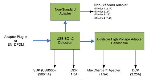
Figure 9. USB D+/D- Detection
