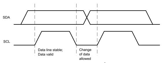
Figure 17. Bit Transfer on the I<sup>2</sup>C Bus
