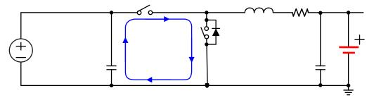
Figure 60. High Frequency Current Path
