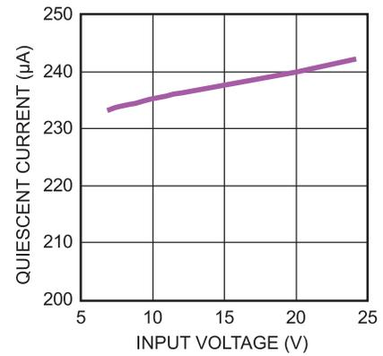
**Supply Current( No Load ) vs. Input Voltage**
