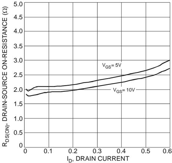
Fig. 3 Typical On-Resistance vs. Drain Current and Temperature
