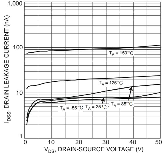
Fig. 8 Typical Drain-Source Leakage Current vs. Voltage
