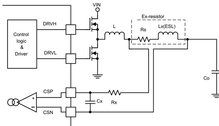
Figure 43. External Resistor Current Sensing
