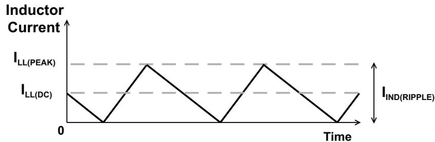
Figure 40. Boundary Between Pulse Skipping and CCM
