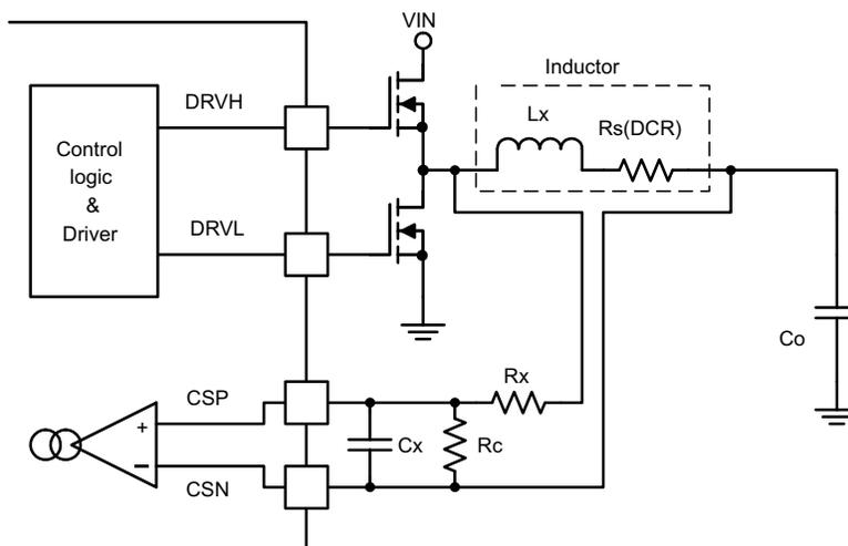
**Figure 45. Inductor DCR Current Sensing With Voltage Divider**
