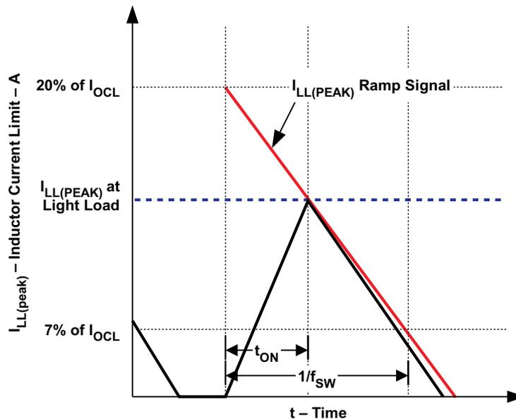
Figure 41. Inductor Current Limit at Pulse Skipping
