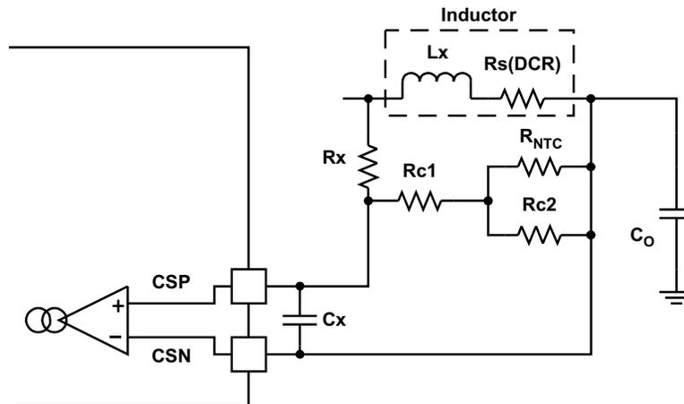
Figure 46. Inductor DCR Current Sensing With Temperature Compensate
