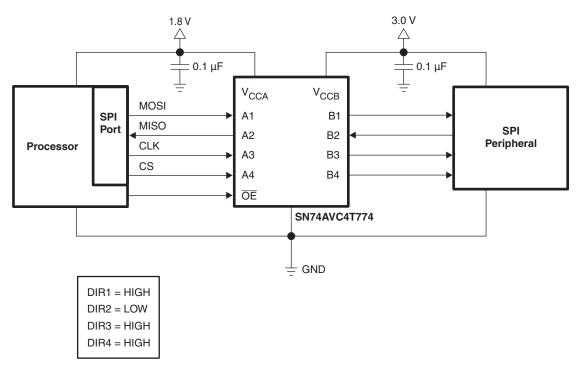
Figure 1. Typical Application of the SN74AVC4T774
