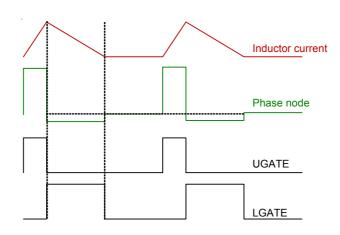
Figure 2. Diode Emulation Mode (DEM) in Steady State
