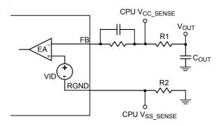
Figure 19. Remote Sensing Circuit
