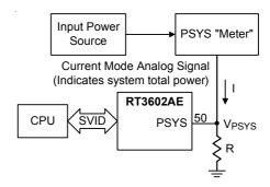
Figure 20. PSYS Function Block Diagram
