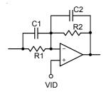
Figure 18. Type I compensator
