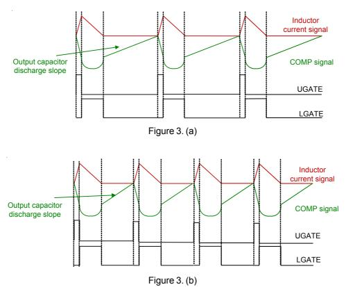
Figure 3. G-NAVP<sup>™</sup> Operation in DEM. (a) : The load is lighter, output capacitor discharge slope is smaller and the switching frequency is lower. (b) : The load is increasing, output capacitor discharge slope is increased and switching frequency is increased, too.
