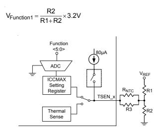
Figure 6. Multi-Function Pin Setting Mechanism for TSEN\_MAIN and TSEN\_AUXI
