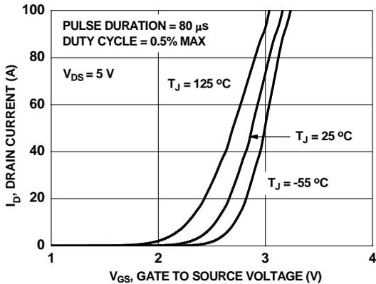
**Figure 5. Transfer Characteristics**
