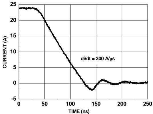
Figure 14. FDMS0308AS SyncFET body diode reverse recovery characteristic
