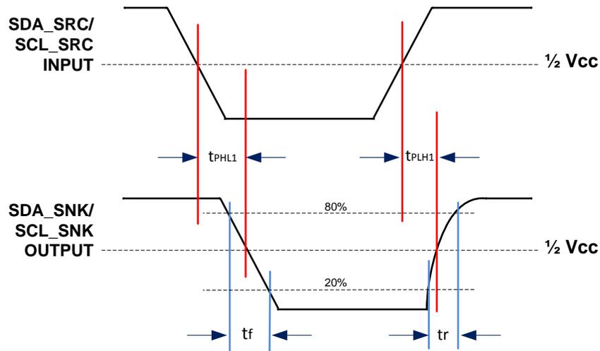
**Figure 15. DDC Propagation Delay – Source to Sink**
