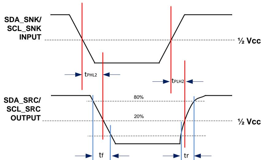
**Figure 16. DDC Propagation Delay – Sink to Source**
