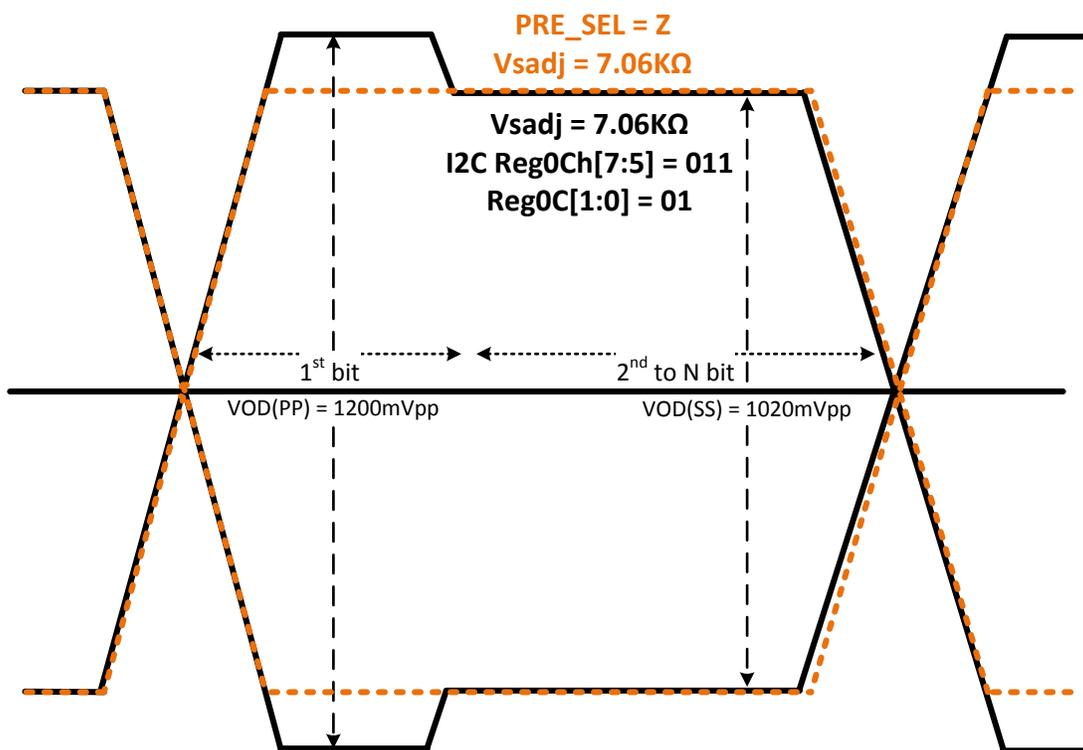
Figure 29. Pre-Emphasis Using I<sup>2</sup>C Method
