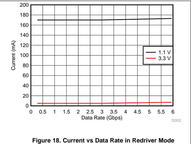
Figure 18. Current vs Data Rate in Redriver Mode
