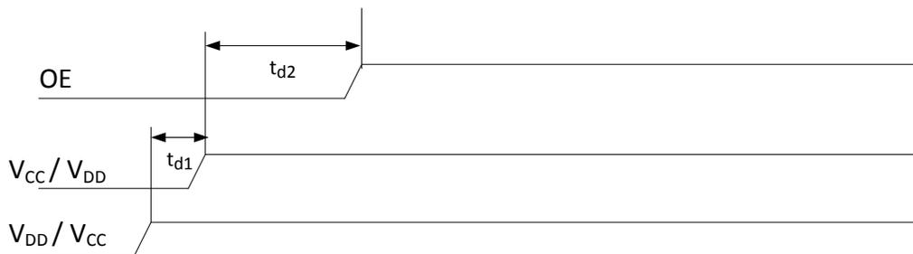
Figure 22. Power-Up Timing for SNx5DP159
