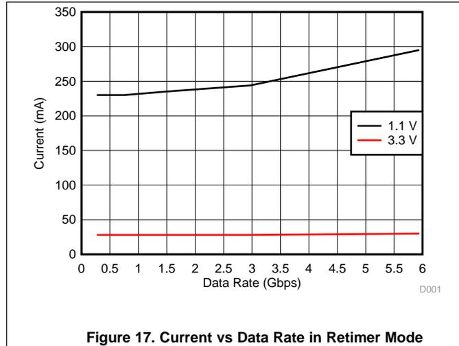
Figure 17. Current vs Data Rate in Retimer Mode
