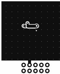
a. 53  $^\circ\text{C}/\text{W}$  when mounted on a 1 in<sup>2</sup> pad of 2 oz copper
