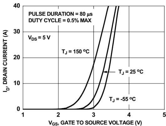
**Figure 5. Transfer Characteristics**
