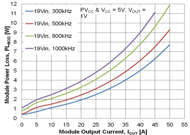
**Figure 7. Power Loss vs. Output Current with 19 V<sub>IN</sub>**
