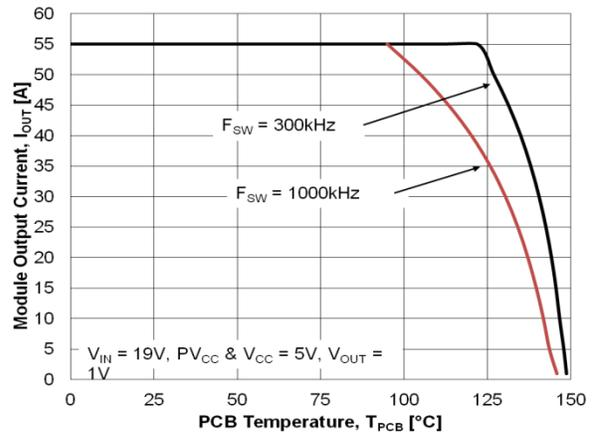
**Figure 5. Safe Operating Area with 19 V<sub>IN</sub>**
