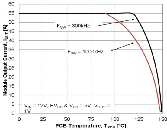
**Figure 4. Safe Operating Area with 12 V<sub>IN</sub>**
