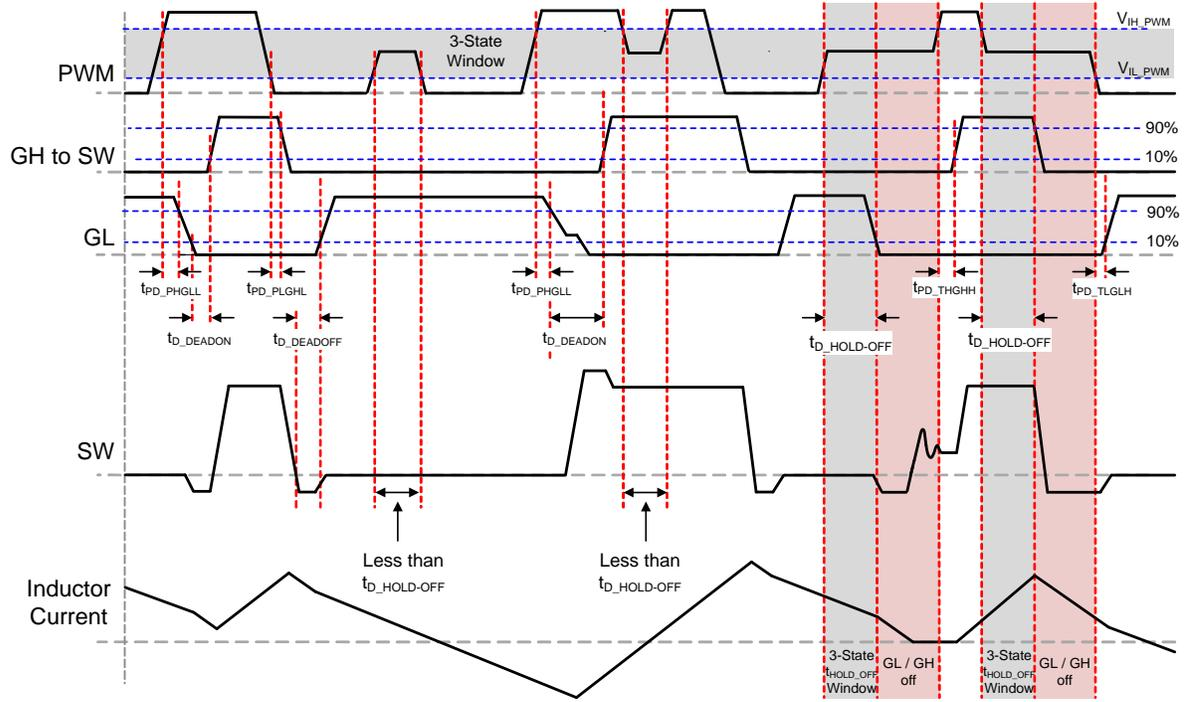
Figure 28. PWM 3-State Timing Diagram (FCCM held HIGH)
