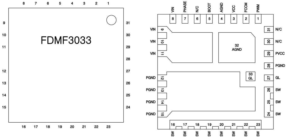
Figure 3. Pin Configuration - Top View and Transparent View
