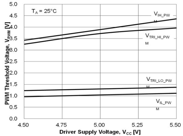
Figure 17. PWM Threshold vs. Driver Supply Voltage
