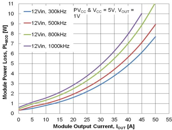
**Figure 6. Power Loss vs. Output Current with 12 V<sub>IN</sub>**
