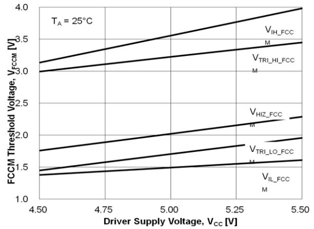
Figure 19. FCCM Threshold vs. Driver Supply Voltage
