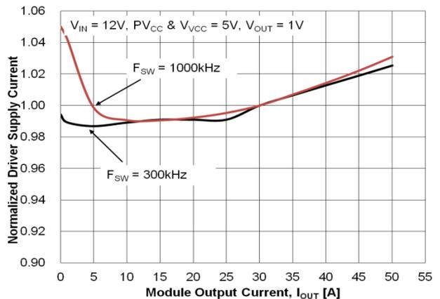
Figure 15. Driver Supply Current vs. Output Current
