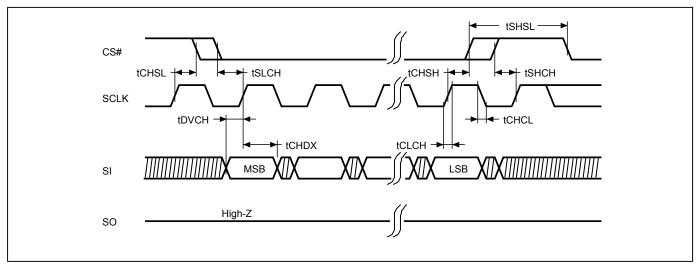
Figure 8. Output Timing
