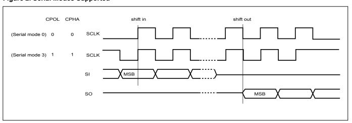
Figure 2. Serial Modes Supported
