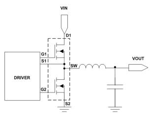
Figure 1. Typical Application Circuit
