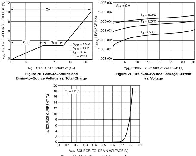
Figure 22. Diode Forward Voltage vs. Current
