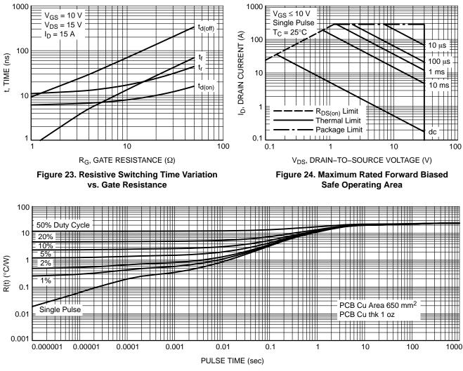
Figure 25. Thermal Characteristics
