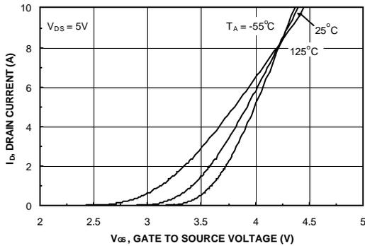
Figure 5. Transfer Characteristics.
