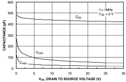
Figure 8. Capacitance Characteristics.
