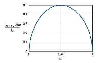
Figure 4. I<sub>CIN</sub> vs. Voltage Conversion Ratio
