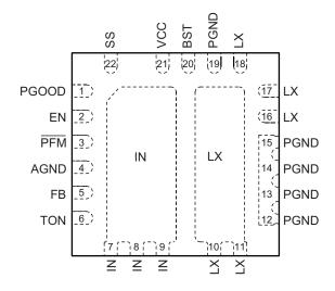
22-Pin 4mm x 4mm QFN (Top View)
