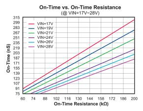
Figure 3. T<sub>ON</sub> vs R<sub>TON</sub> Curves for AOZ2261QI-11
