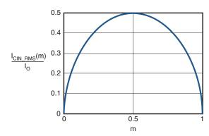
Figure 2. I<sub>CIN</sub> vs. Voltage Conversion Ratio
