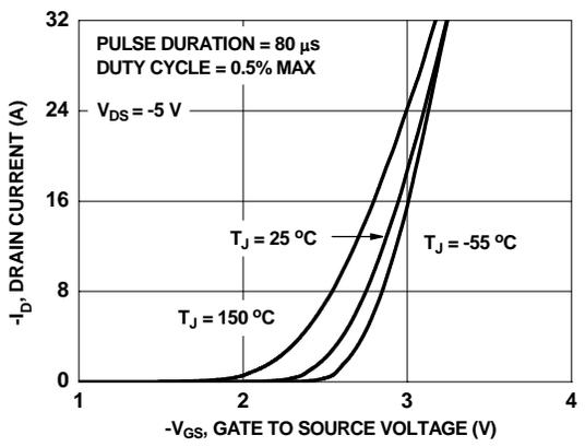
**Figure 5. Transfer Characteristics**
