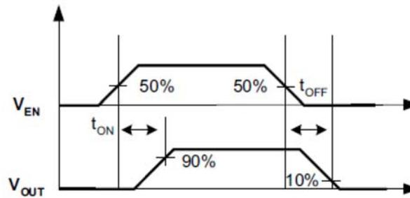
Response Time to Short-Circuit Waveforms
