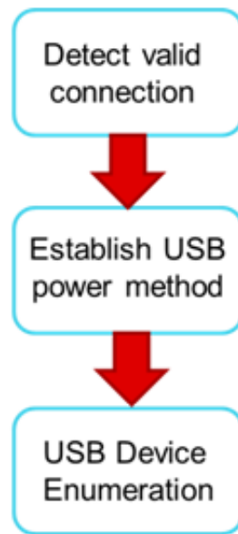
Figure 11. Flow of DFP to UFP Configuration
