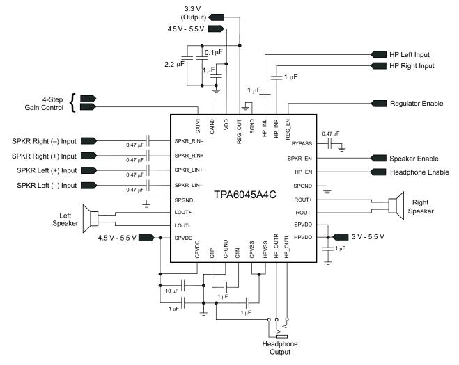
Figure 39. Differential Input Application Circuit
