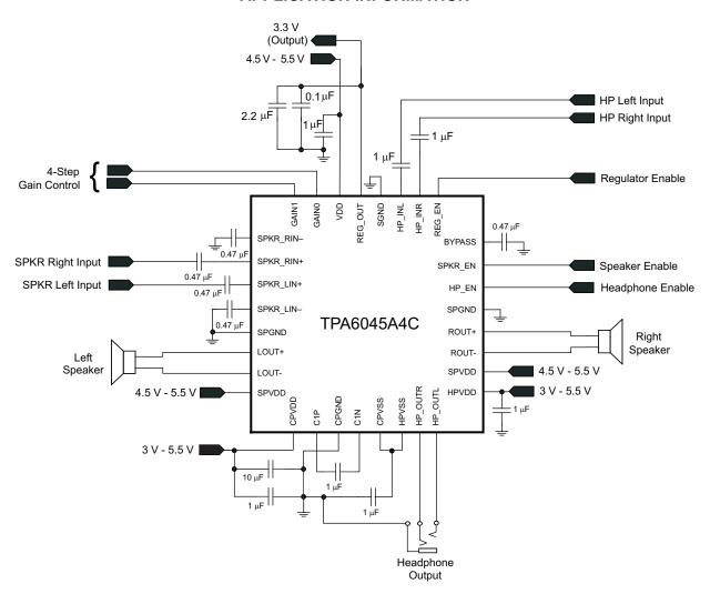
Figure 38. Single-Ended Input Application Circuit
