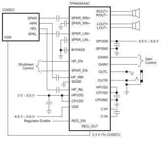
The TPA6045A4C is a stereo audio power amplifier and DirectPath™ headphone amplifier in a thermally enhanced, space-saving, 32-pin QFN package. The speaker amplifier is capable of driving 2.1 W per channel continuously into 4-Ω loads at 5 V. The headphone amplifier achieves a minimum of 85 mW at 1% THD+N from a 5-V supply. A built-in internal 4-step gain control for the speaker amplifier and a fixed −1.5 V/V gain for the headphone amplifier minimizes external components needed.
