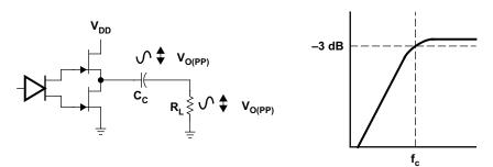
Figure 42. Single-Ended Configuration and Frequency Response
