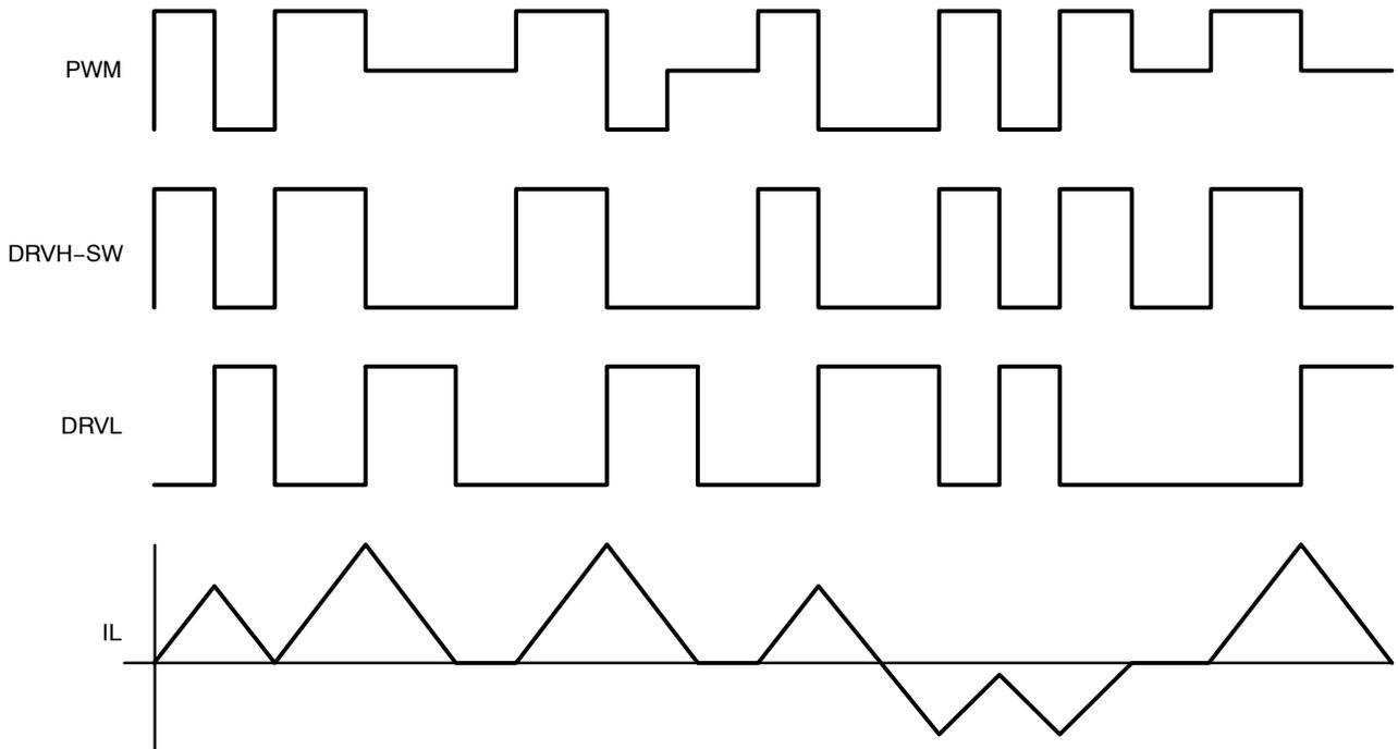
Figure 5. Timing Diagram
