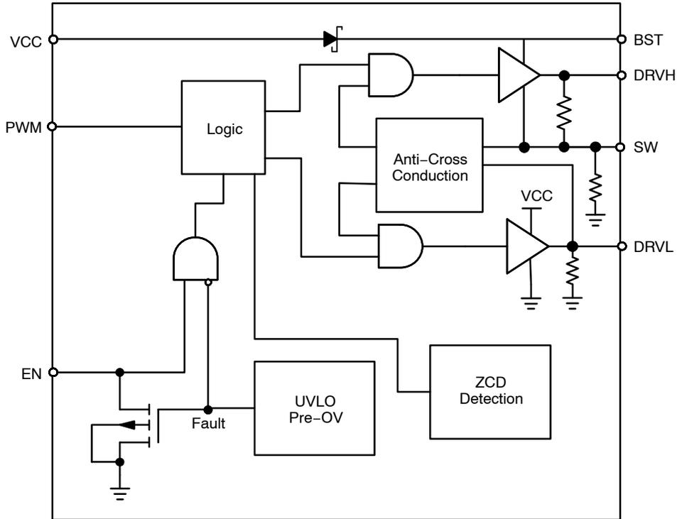
Figure 2. Block Diagram
