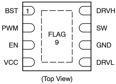
Figure 1. Pin Diagram
