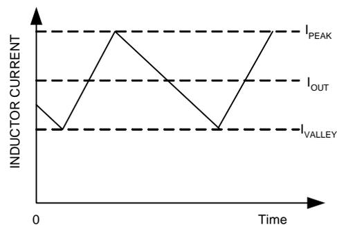
Figure 2. Over-Current Algorithm
