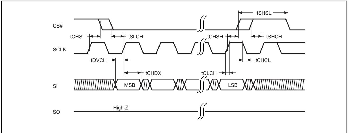
**Figure 8. Output Timing**
