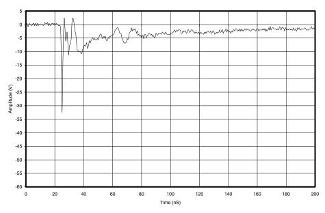
Figure 5. IEC Clamping Waveforms –8 kV Contact, 1 GHz Bandwidth
