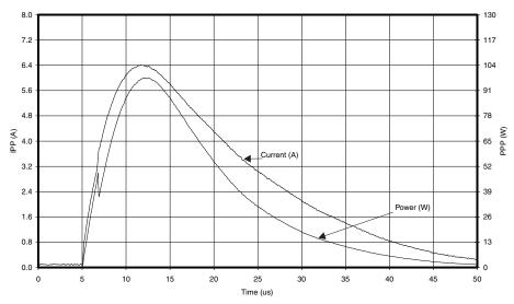
Figure 3. Peak Pulse Waveforms Ch2\_In, PUT wrt GND,  $V_{\rm CC}$  = 5.0 V
