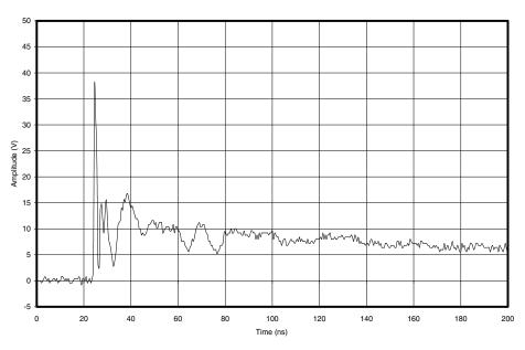
Figure 4. IEC Clamping Waveforms 8 kV Contact, 1 GHz Bandwidth
