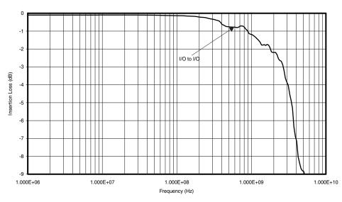
Figure 1. Insertion Loss Data (S21)
