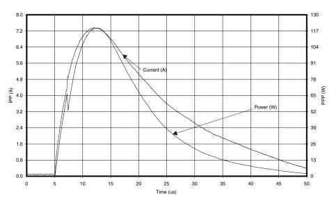
Figure 2. Peak Pulse Waveforms Ch1\_Out, PUT wrt GND,  $V_{CC} = 5.0 \text{ V}$
