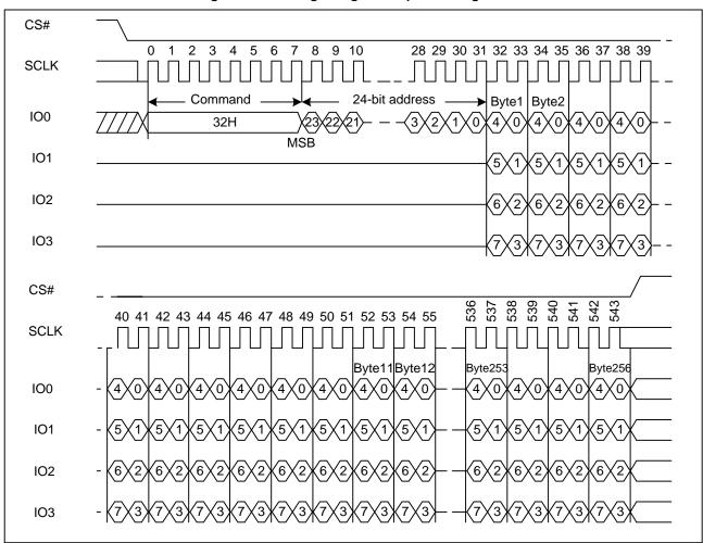
Figure 15. Quad Page Program Sequence Diagram
