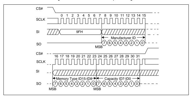
Figure 24. Read Identification ID Sequence Diagram
