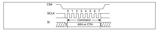
Figure19a. Chip Erase Sequence Diagram (QPI)
