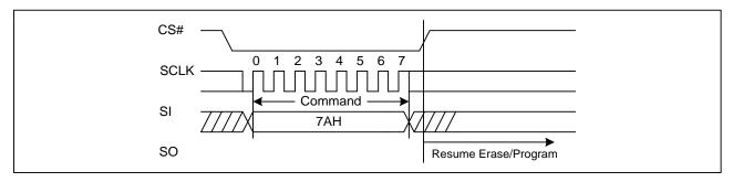
Figure 26a. Program/Erase Resume Sequence Diagram (QPI)
