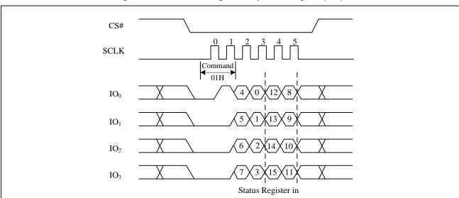
Figure6a. Write Status Register Sequence Diagram (QPI)
