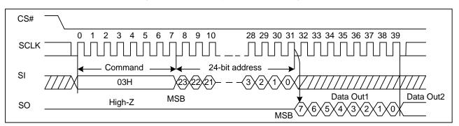
Figure 7. Read Data Bytes Sequence Diagram
