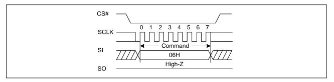
Figure 2. Write Enable Sequence Diagram (QPI)
