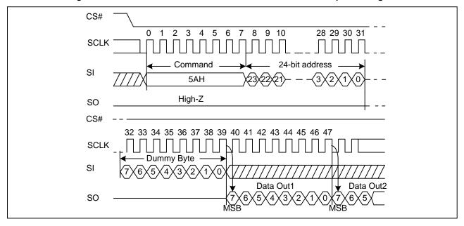
Figure 36a. Read Serial Flash Discoverable Parameter command Sequence Diagram (QPI)
