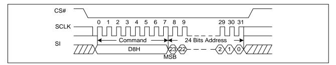
Figure 18a. 64KB Block Erase Sequence Diagram (QPI)
