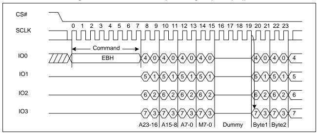
Figure 12. Quad I/O Fast Read Sequence Diagram (M5-4≠ (1, 0))
