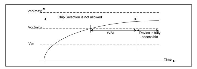
Table7. Power-Up Timing And Write Inhibit Threshold
