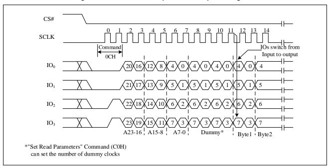
Figure 32. Burst Read with Wrap command Sequence Diagram
