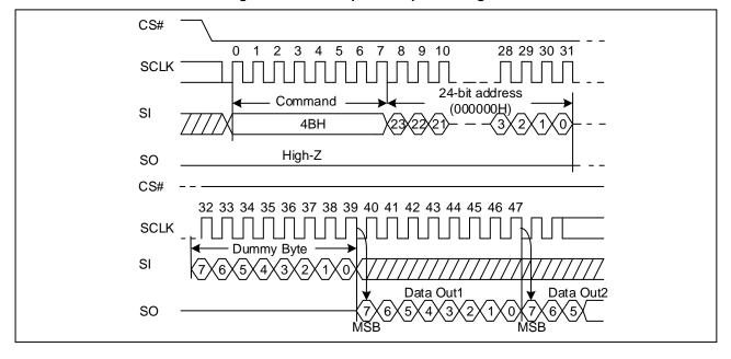
Figure 27. Read Unique ID Sequence Diagram
