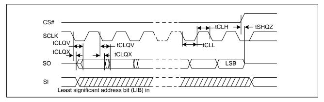
Figure 41. Resume to Suspend Timing Diagram
