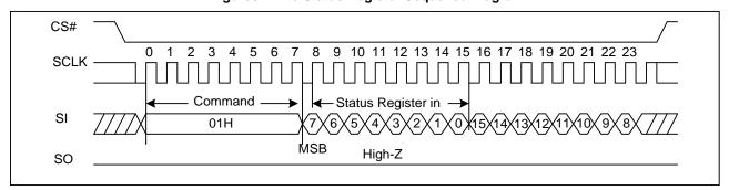
Figure 6. Write Status Register Sequence Diagram
