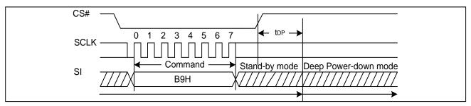
Figure 20a. Deep Power-Down Sequence Diagram (QPI)
