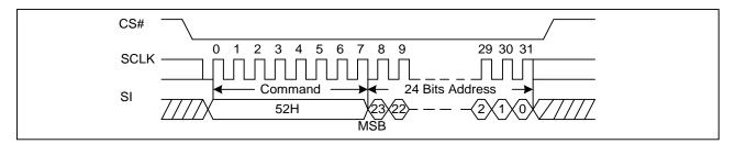
Figure 17a. 32KB Block Erase Sequence Diagram (QPI)
