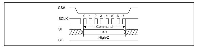
Figure3a. Write Disable Sequence Diagram (QPI)
