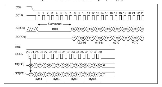
Figure11a. Dual I/O Fast Read Sequence Diagram (M5-4= (1, 0))
