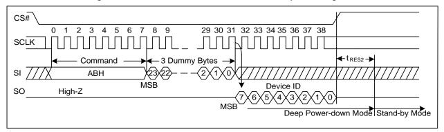
Figure22a. Release Power-Down/Read Device ID Sequence Diagram (QPI)
