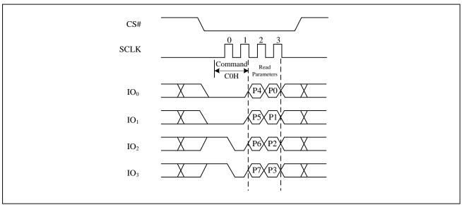
Figure 31. Set Read Parameters command Sequence Diagram
