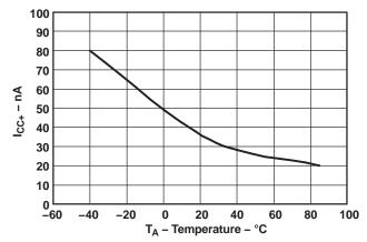
Figure 9. Power-Supply Current vs Temperature (V<sub>+</sub> = 5 V)
