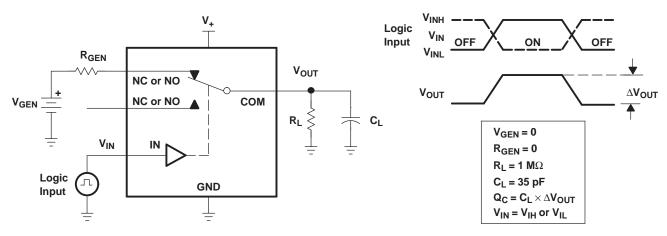
Figure 18. Charge Injection (Q<sub>C</sub>)
