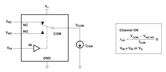
Figure 10. ON-State Resistance on)
