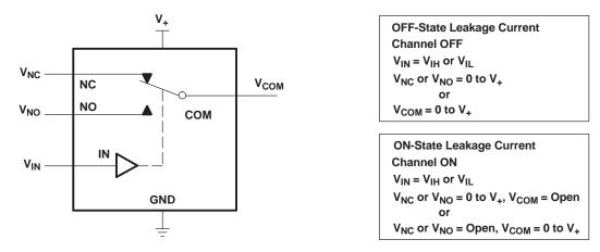
Figure 11. ON- and OFF-State Leakage Current ( $I_{COM(ON)}$ ,  $I_{NC(OFF)}$ ,  $I_{NO(OFF)}$ ,  $I_{NO(ON)}$ )
