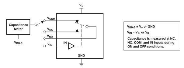
Figure 12. Capacitance IN, C<sub>COM(ON)</sub>, C<sub>NC(OFF)</sub>, C<sub>NO(OFF)</sub>, C<sub>NC(ON)</sub>, C<sub>NO(ON)</sub>)
