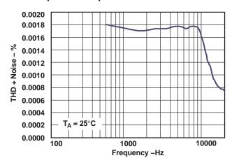
Figure 7. Frequency Response (V<sub>+</sub> = 3 V)
