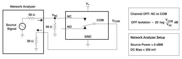
Figure 16. OFF Isolation (O<sub>ISO</sub>)
