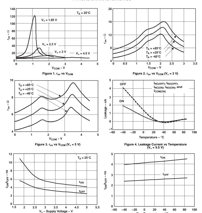
Figure 5.  $t_{ON}$  and  $t_{OFF}$  vs  $V_{+}$
