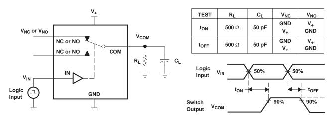
Figure 13. Turn-On (t<sub>ON</sub>) and Turn-Off (t<sub>OFF</sub>) Time
