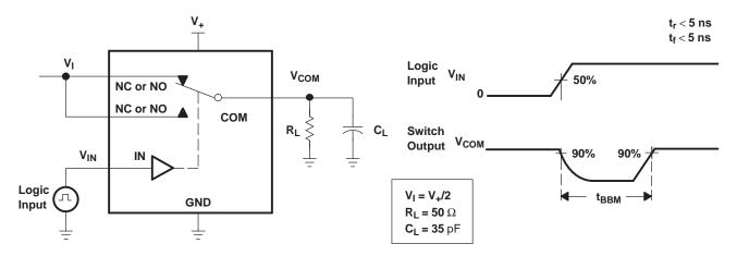
Figure 14. Break-Before-Make (t<sub>BBM</sub>) Time
