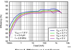
Figure 5. Efficiency vs Load Current
