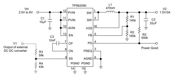
Figure 28. Output Voltage Tracking
