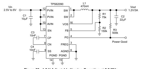
Figure 29. 1.2 V Adjustable Version Operating at 2.8 MHz
