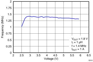
Figure 12. Switching Frequency vs Input Voltage
