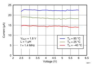
Figure 15. Quiescent Current vs Input Voltage
