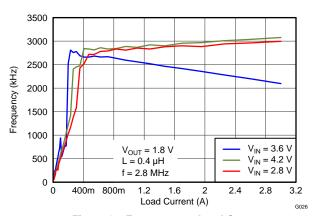
Figure 13. Frequency vs Load Current
