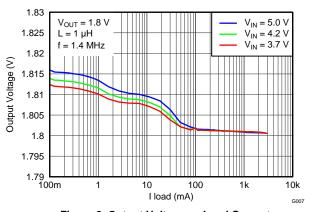
Figure 8. Output Voltage vs Load Current
