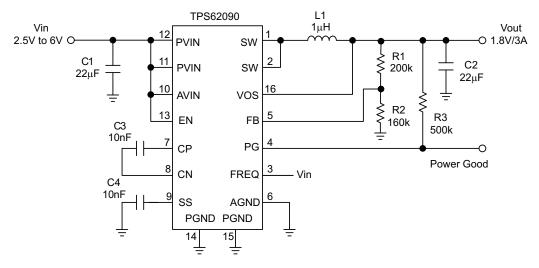
Figure 31. 1.8 V Adjustable Version Operating at 1.4 MHz
