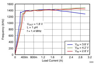
Figure 11. Switching Frequency vs Load Current
