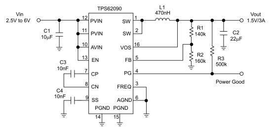
Figure 30. 1.5 V Adjustable Version Operating at 2.8 MHz
