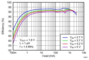
Figure 4. Efficiency vs Load Current
