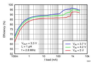
Figure 3. Efficiency vs Load Current
