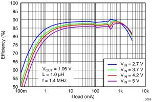
Figure 6. Efficiency vs Load Current
