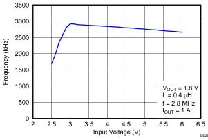
Figure 14. Frequency vs Input Voltage
