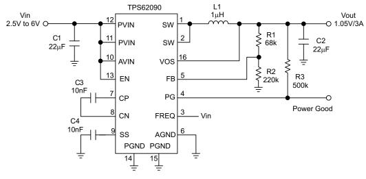
Figure 32. 1.05 V Adjustable Version Operating at 1.4 MHz
