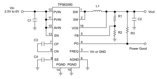
**Figure 1. Parametric Measurement Circuit**
