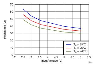
Figure 10. High Side FET On-Resistance vs Input Voltage
