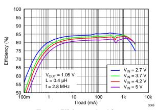
Figure 7. Efficiency vs Load Current
