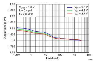
Figure 9. Output Voltage vs Load Current
