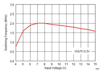
Figure 8. Typical Switching Frequency vs Input Voltage
