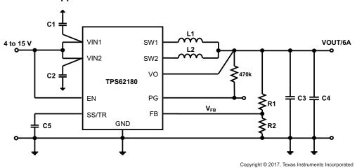
Figure 10. Typical 4-V to 15-V Input, 6A Converter
