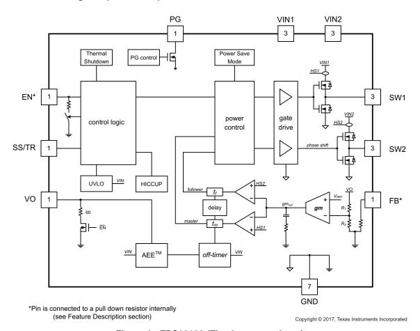
Figure 6. TPS62182 (Fixed output voltage)
