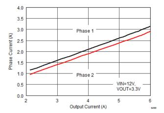
Figure 9. Typical Current Balancing vs Load Current
