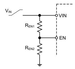
Figure 40. Resistive Divider for Controlled EN Threshold
