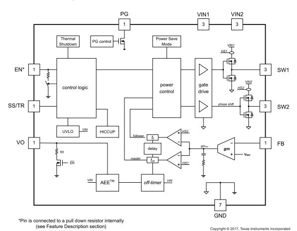
Figure 5. TPS62180 (Adjustable output voltage)
