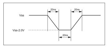
**Figure 4. Maximum Positive Overshoot Waveform**
