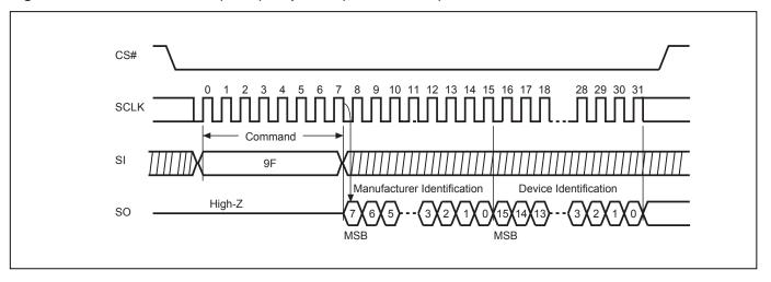
Figure 26. Read Electronic Manufacturer & Device ID (REMS) Sequence (Command 90)
