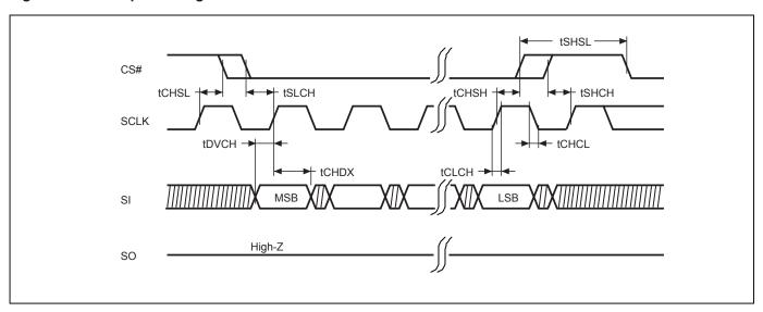
Figure 8. Output Timing
