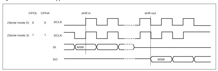
Figure 1. Serial Modes Supported
