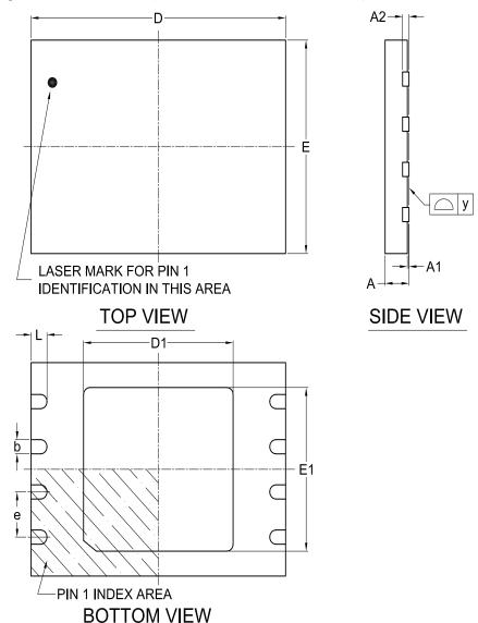
Dimensions (inch dimensions are derived from the original mm dimensions)
