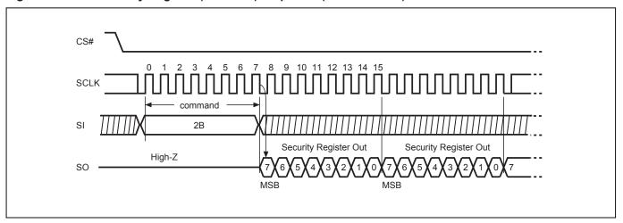
Figure 28. Write Security Register (WRSCUR) Sequence (Command 2F)
