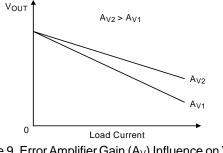
Figure 9. Error Amplifier Gain (A<sub>V</sub>) Influence on  $V_{OUT}$ Accuracy
