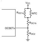
Figure 15. OCP Setting with Temperature Compensation
