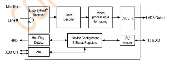
Figure 1: ANX3112 Block Diagram
