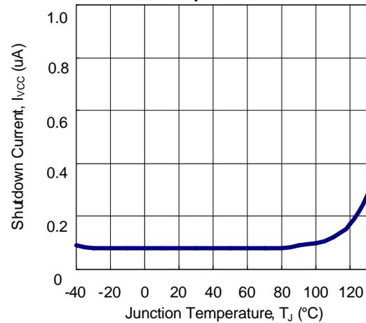
Supply Current in S3 State vs. Junction Temperature
