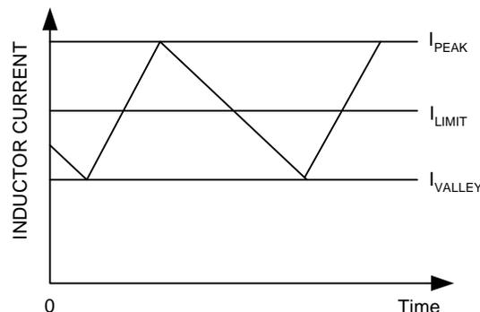
Figure 2. Current-Limit Algorithm
