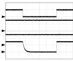
CH1:  $V_{S3}$  (5V/div) CH2:  $V_{VDDQ}$  (1V/div) CH3:  $V_{VTTREF}$  (500mV/div) CH4:  $V_{VTT}$  (500mV/div) Time: 10ms/div
