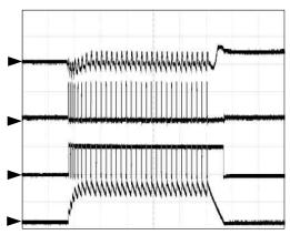
CH1:  $V_{VDDQ}$  (100mV/div) CH2:  $V_{UGATE}$  (20V/div) CH3:  $V_{LGATE}$  (5V/div) CH4:  $I_L$  (10A/div) Time: 20 $\mu$ s/div
