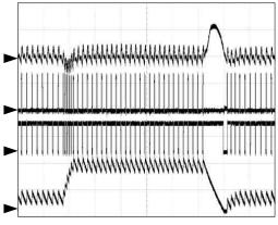
$\begin{array}{l} CH1: V_{VDDQ} \ (100mV/div) \\ CH2: V_{UGATE} \ (20V/div) \\ CH3: V_{LGATE} \ (5V/div) \\ CH4: I_L \ (10A/div) \\ Time: 20\mus/div \end{array}$
