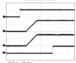
CH1:  $V_{SS}$  (5V/div) CH2:  $V_{VDDQ}$ (1V/div) CH3:  $V_{VTT}$  (500mV/div) CH4:  $V_{POK}$  (5V/div) Time: 500 $\mu$ s/div
