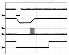
$\begin{array}{l} \text{CH1: V}_{\text{S5}}\left(5\text{V/div}\right) \\ \text{CH2: V}_{\text{VDDQ}}\left(1\text{V/div}\right) \\ \text{CH3: V}_{\text{UGATE}}\left(20\text{V/div}\right) \\ \text{CH4: V}_{\text{POK}}\left(5\text{V/div}\right) \\ \text{Time: } 500\mu\text{s/div} \end{array}$
