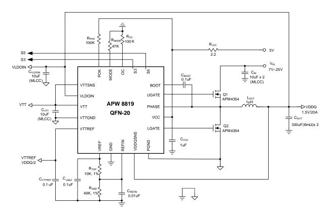
DDR3, 400kHz Application Circuit
