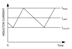
Figure 2. Current-Limit Algorithm
