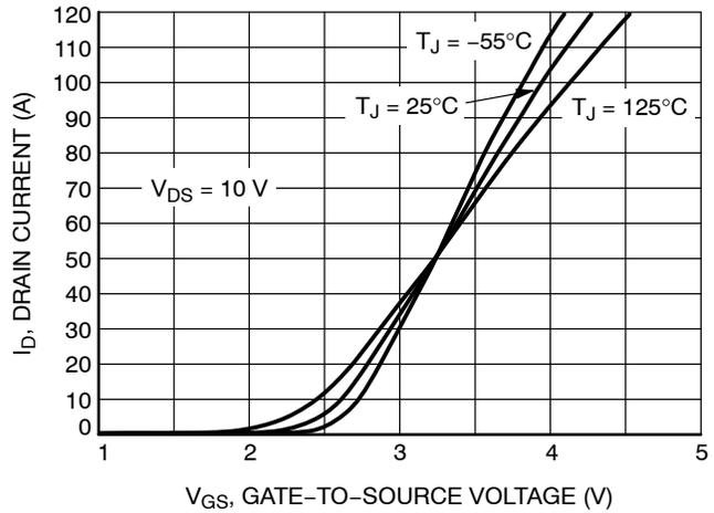
Figure 2. Transfer Characteristics
