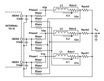
FIGURE 12. DIFFERENTIAL-SENSING CURRENT BALANCING CIRCUIT
