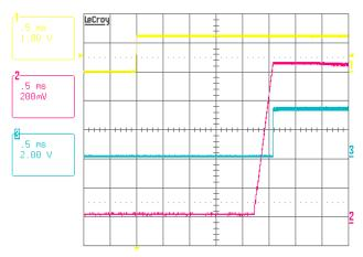
FIGURE 30. VR1 SOFT-START,  $V_{\rm IN}$  = 19V,  $I_{\rm O}$  = 5A, VID = 1.1V, CH1: VR\_ON, CH2: VR1  $V_{\rm O}$ , CH3: PGOOD
