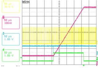
FIGURE 45. VR1 SETVID-SLOW RESPONSE, I $_0$  = 5A, VID = 0.3V - 0.9V, CH1: PHASE1, CH2: VR1 V $_0$ , CH3: SDA, CH4: ALERT#
