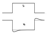
FIGURE 19. LOAD TRANSIENT RESPONSE WHEN  $\mathbf{C_n}$  IS TOO SMALL
