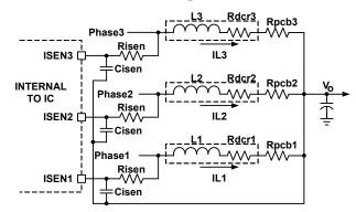
FIGURE 11. CURRENT BALANCING CIRCUIT
