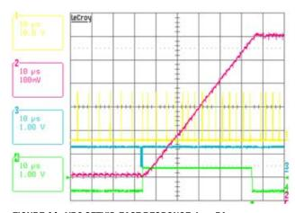
FIGURE 44. VR2 SETVID-FAST RESPONSE, I $_0$  = 5A, VID = 0.5V - 0.8V, CH1: PHASE1G, CH2: VR2 V $_0$ , CH3: SDA, CH4: ALERT#
