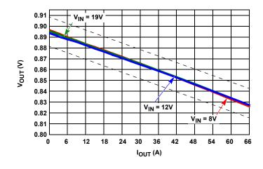
FIGURE 2. LOAD LINE REGULATION
