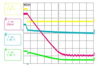
FIGURE 34. VR1 SHUT DOWN,  $V_{IN}$  = 12V,  $I_{O}$  = 5A, VID = 1.1V, CH1: PG00D, CH2: VR1  $V_{O}$ , CH3: VR\_ON, CH4: COMP
