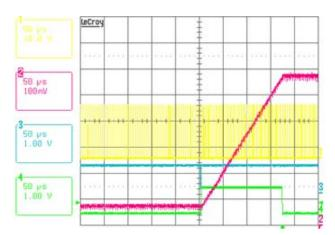
FIGURE 46. VR2 SETVID-SLOW RESPONSE,  $I_0$  = 5A, VID = 0.4V - 0.9V, CH1: PHASE1G, CH2: VR2 V<sub>0</sub>, CH3: SDA, CH4: ALERT#
