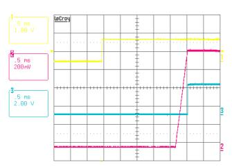
FIGURE 31. VR2 SOFT-START,  $V_{IN}$  = 19V,  $I_{O}$  = 5A, VID = 1.1V, CH1: VR\_ON, CH2: VR2  $V_{O}$ , CH3: PGOODG
