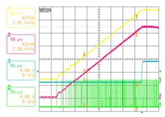
FIGURE 33. 1 VR1 AND VR2 SOFT-START,  $V_{\rm IN}$  = 20V,  $I_{\rm O\_VR1}$  = 30A,  $I_{\rm O\_VR2}$  = 30A, VID = 1.1V, CH1: VR1  $V_{\rm O}$ , CH2: VR2  $V_{\rm O}$ , CH3: PGOOD, CH4: PHASE1G
