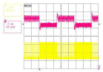
FIGURE 41. VR1 PS2 LOAD TRANSIENT RESPONSE,  $V_{IN}$  = 19V, VID = 0.6V,  $I_0$  = 1A/5A, SLEW TIME= 150ns, LL = 1.9m $\Omega$ , CH1: PHASE1, CH2: VR1  $V_0$
