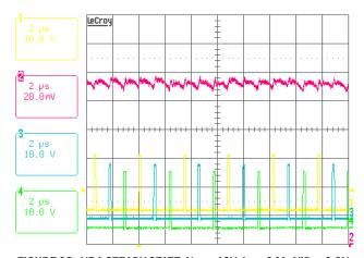
FIGURE 38. VR1 STEADY STATE,  $V_{IN} = 19V$ ,  $I_0 = 94A$ , VID = 0.9VCH1: PHASE1, CH2: VR1 VO. CH3: PHASE2, CH4: PHASE3
