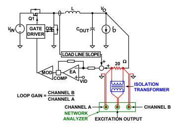
FIGURE 26. LOOP GAIN T2(s) MEASUREMENT SET-UP
