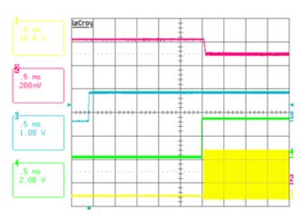
FIGURE 37. VR2 PRE-CHARGED START UP, VIN = 19V, VID = 1.1V, **V\_PRE-CHARGE VOLTAGE = 1.3V, CH1: PHASE1G,** CH2: VR2 V<sub>0</sub>, CH3: VR\_ON, CH4: PGOODG
