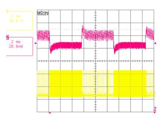
FIGURE 42. VR2 PS2 LOAD TRANSIENT RESPONSE,  $v_{IN}$  = 19V, VID = 0.6V,  $v_{IO}$  = 1A/5A, SLEW TIME= 150ns, LL = 3.9m $v_{IO}$ , CH1: PHASE1G, CH2: VR2  $v_{IO}$
