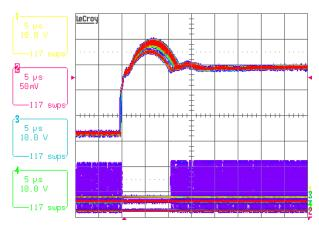
FIGURE 39. VR1 LOAD RELEASE RESPONSE, VIN = 12V, VID = 0.9V,  $I_0 = 28A/94A$ , SLEW TIME= 150ns, LL = 1.9m $\Omega$ , CH1: PHASE1, CH2: VR1 V<sub>0</sub>, CH3: PHASE2, CH4: PHASE3
