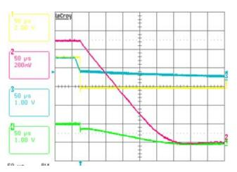
FIGURE 35. VR2 SHUT DOWN,  $V_{\rm IN}$  = 12V,  $I_{\rm O}$  = 5A, VID = 1.1V, CH1: PG00DG, CH2: VR2  $V_{\rm O}$ , CH3: VR\_ON, CH4: COMPG
