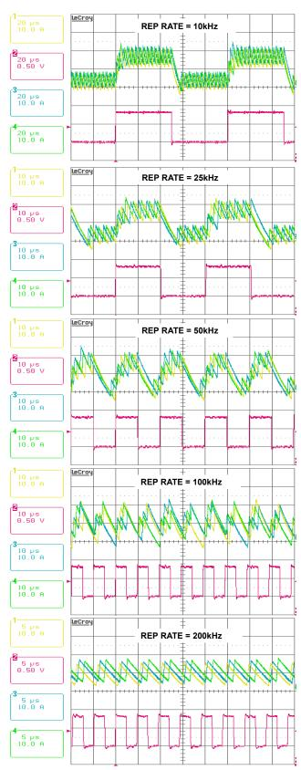
FIGURE 13. CURRENT BALANCING DURING DYNAMIC OPERATION. CH1: IL1, CH2: IL0AD, CH3: IL2, CH4: IL3
