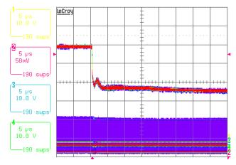
FIGURE 40. VR1 LOAD INSERTION RESPONSE,  $V_{IN} = 12V$ , VID = 0.9V,  $I_0 = 28A/94A$ , SLEW TIME= 150ns,  $LL = 1.9m\Omega$ , CH1: PHASE1, CH2: VR1 V<sub>0.</sub> CH3: PHASE2, CH4: PHASE
