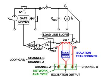
FIGURE 25. LOOP GAIN T1(s) MEASUREMENT SET-UP
