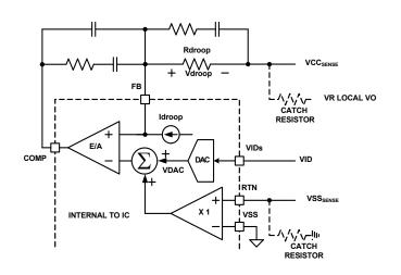
FIGURE 10. DIFFERENTIAL SENSING AND LOAD LINE IMPLEMENTATION
