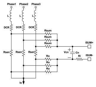
FIGURE 23. RESISTOR CURRENT-SENSING NETWORK
