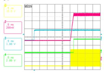
FIGURE 36. VR1 PRE-CHARGED START UP, VIN = 19V, VID = 1.1V, V\_PRE-CHARGE VOLTAGE = 0.5V, CH1: PHASE1, CH2: VR1 V<sub>0</sub>, CH3: VR\_ON, CH4: PGOOD
