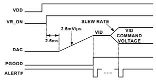
FIGURE 9. VR1 SOFT-START WAVEFORMS
