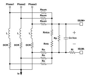
FIGURE 17. DCR CURRENT-SENSING NETWORK
