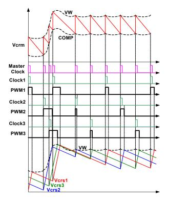
FIGURE 6. R3<sup>™</sup> MODULATOR OPERATION PRINCIPLES IN LOAD INSERTION RESPONSE
