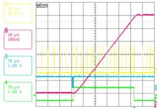
FIGURE 43. VR1 SETVID-FAST RESPONSE, I  $_0$  = 5A, VID = 0.3V - 0.9V, CH1: PHASE1, CH2: VR1 V $_0$ , CH3: SDA, CH4: ALERT#
