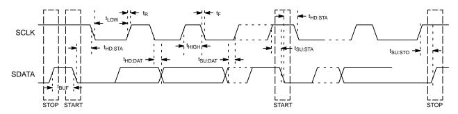
Figure 3. I<sup>2</sup>C Timing Diagram
