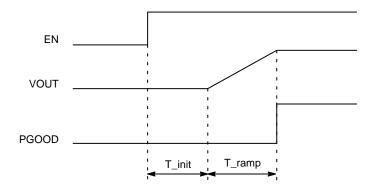
Figure 4. Soft Start Timing Diagram
