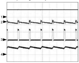
CH1:  $V_{PGOOD}$  (5V/div) CH2:  $V_{OUT1}$  (AC, 100mV/div) CH3:  $V_{PHASE}$  (10V/div) CH4:  $I_L$  (5A/div) Time:  $2\mu$ s/div
