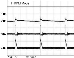
CH1: V<sub>PGOOD</sub> (5V/div) CH2: V<sub>OUT1</sub> (AC, 100mV/div) CH3: V<sub>PHASE</sub> (10V/div) CH4: I<sub>L</sub> (2A/div) Time: 20us/div
