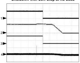
$\begin{array}{c} \text{CH1: V}_{\text{EN}} \text{ (5V/div)} \\ \text{CH2: V}_{\text{OUT}} \text{ (1V/div)} \\ \text{CH3: V}_{\text{PGOOD}} \text{ (5V/div)} \\ \text{CH4: V}_{\text{PHASE}} \text{ (10V/div)} \\ \text{Time: 5ms/div} \end{array}$
