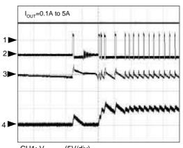
CH1: V<sub>PGOOD</sub> (5V/div) CH2: V<sub>PHASE</sub> (10V/div) CH3: V<sub>OUT</sub> (AC, 100mV/div) CH4: I<sub>L</sub> (5A/div) Time: 10µs/div
