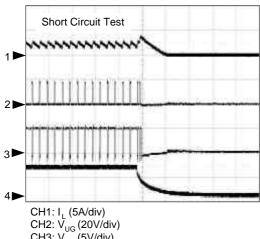
$\begin{array}{c} \text{CH1: I}_{L} \left(5\text{A/div}\right) \\ \text{CH2: V}_{\text{UG}} \left(20\text{V/div}\right) \\ \text{CH3: V}_{\text{LG}} \left(5\text{V/div}\right) \\ \text{CH4: V}_{\text{OUT}} \left(1\text{V/div}\right) \\ \text{Time: } 10\mu\text{s/div} \end{array}$
