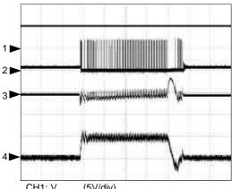
$\begin{array}{l} \text{CH1: V}_{\text{PGOOD}}\left(5\text{V/div}\right) \\ \text{CH2: V}_{\text{PHASE}}\left(10\text{V/div}\right) \\ \text{CH3: V}_{\text{OUT}}\left(\text{AC, 100mV/div}\right) \\ \text{CH4: I}_{\text{L}}\left(5\text{A/div}\right) \\ \text{Time: 50}\mu\text{s/div} \end{array}$
