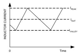
Figure 2. Over-Current Algorithm
