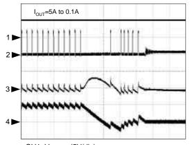
CH1:  $V_{PGOOD}$  (5V/div) CH2:  $V_{PHASE}$  (10V/div) CH3:  $V_{OUT}$  (AC, 100mV/div) CH4:  $I_L$  (5A/div) Time: 10 $\mu$ s/div
