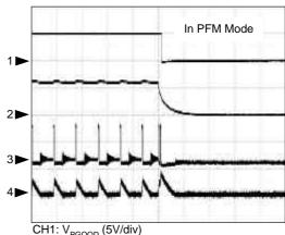
CH1:  $V_{PGOOD}$  (5V/div) CH2:  $V_{OUT}$  (1V/div) CH3:  $V_{PHASE}$  (10V/div) CH4:  $I_{L}$  (5A/div) Time: 20 $\mu$ s/div
