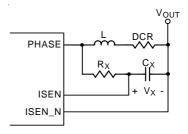
Figure 3. Lossless Inductor Current Sensing
