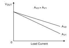
Figure 5. Error Amplifier Gain (Av) Influence on  $V_{\text{OUT}}$
