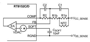
Figure 6. Loop Setting with Temperature Compensation
