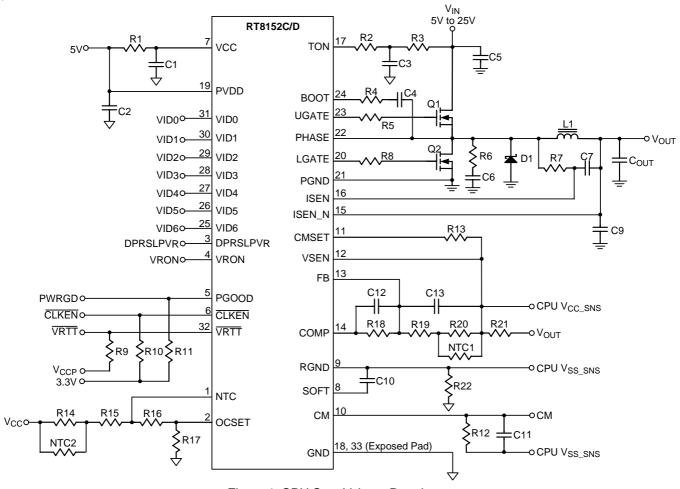
Figure 1. CPU Core Voltage Regulator
