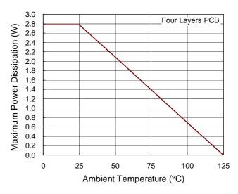
Figure 15. Derating Curve for RT8152C/D Package
