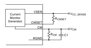
Figure 14. Current Monitor Setting Principle
