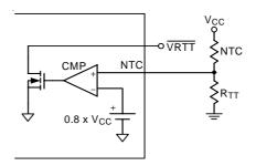
Figure 12. Thermal Throttling Setting Principle
