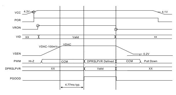
Figure 9. Render Mode Timing Diagram for Power-Up and Power-Down
