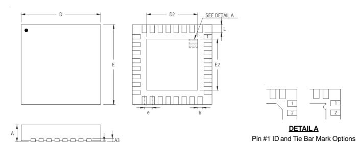
Note: The configuration of the Pin #1 identifier is optional, but must be located within the zone indicated.
