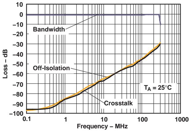
Figure 7. Frequency Response ( $V_+ = 3\text{ V}$ )
