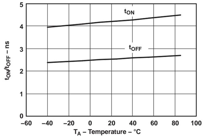
Figure 6.  $t_{ON}$  and  $t_{OFF}$  vs Temperature ( $V_+ = 5$  V)
