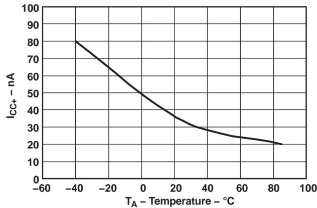
Figure 9. Power-Supply Current vs Temperature ( $V_+ = 5\text{ V}$ )
