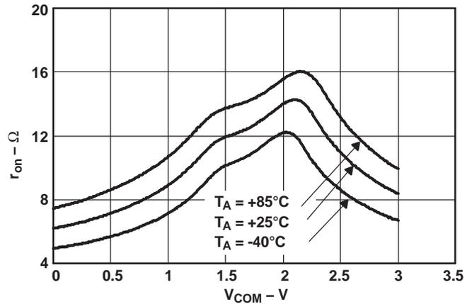
Figure 2.  $r_{on}$  vs  $V_{COM}$  ( $V_+ = 3$  V)
