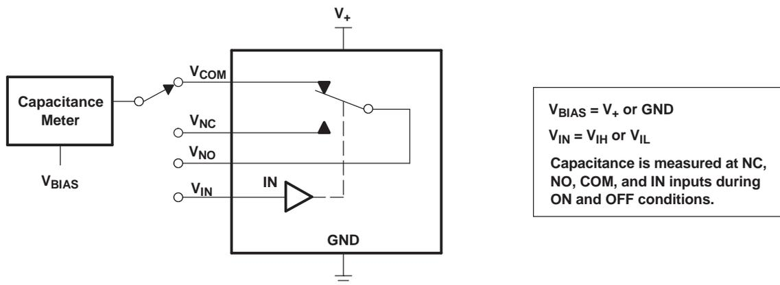
Figure 12. Capacitance  $C_{IN}$ ,  $C_{COM(ON)}$ ,  $C_{NC(OFF)}$ ,  $C_{NO(OFF)}$ ,  $C_{NC(ON)}$ ,  $C_{NO(ON)}$
