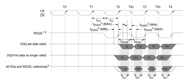
Figure 9. Data Output Timing (1) -  $t_{DQSQ}$ ,  $t_{QH}$  and Data Valid Window
