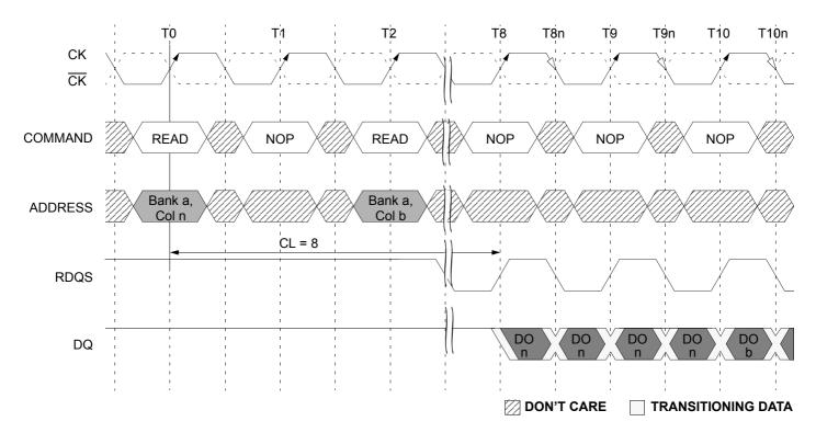
**NOTE**: 1. DO n (or x or b or g) = data-out from column n (or column x or column x or column b or column g).
