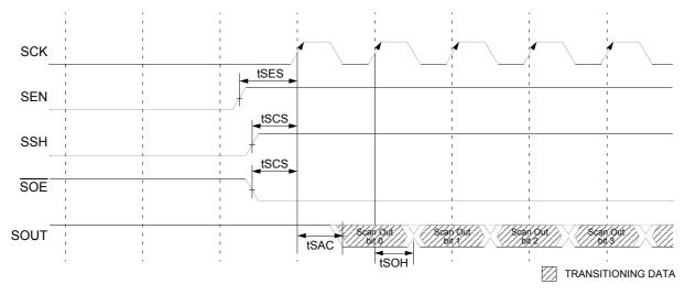
Figure 5. Scan Shift Timing
