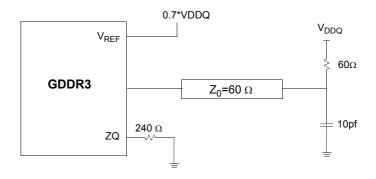
NOTE : 1. Outputs measured into equivalent load of 10pf at a driver impedance of 40  $\Omega$
