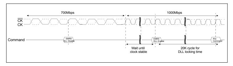
Figure 1. Clock frequency change sequence after the power-up(example)
