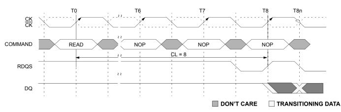
Burst Length = 4 in the cases shown Shown with nominal  $t_{AC}$  and nominal  $t_{DSDQ}$
