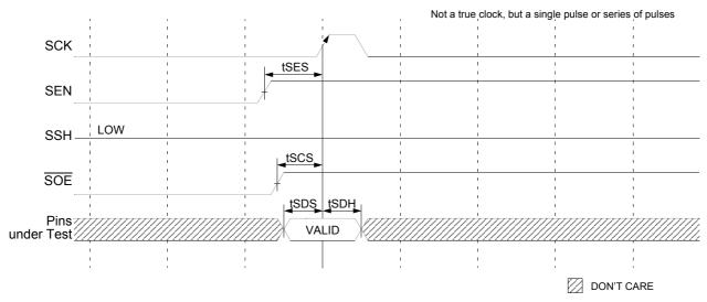
Figure 4. Scan Capture Timing
