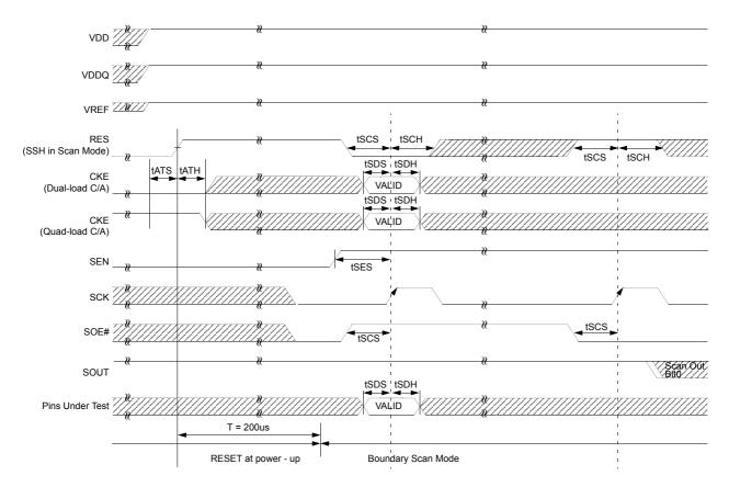
NOTE: To set the pre-defined ODT for C/A, a boundary scan mode should be issued after an appropriate ODT initialization sequence with RES and CKE signals
