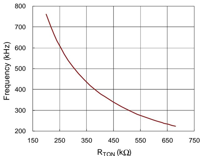
Figure 5. Frequency vs. R<sub>TON</sub>
