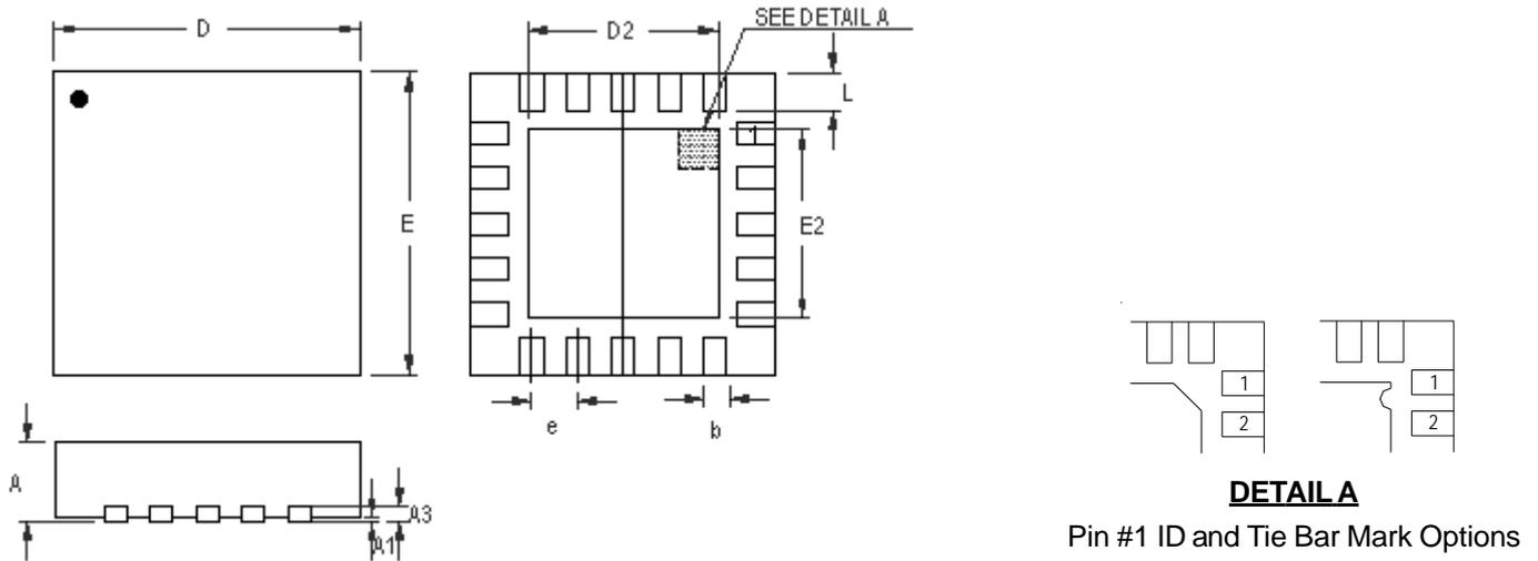
Note : The configuration of the Pin #1 identifier is optional, but must be located within the zone indicated.
