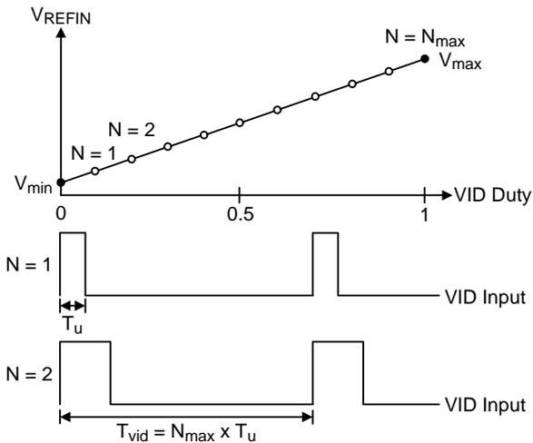
Figure 10. PWM VID Analog Output
