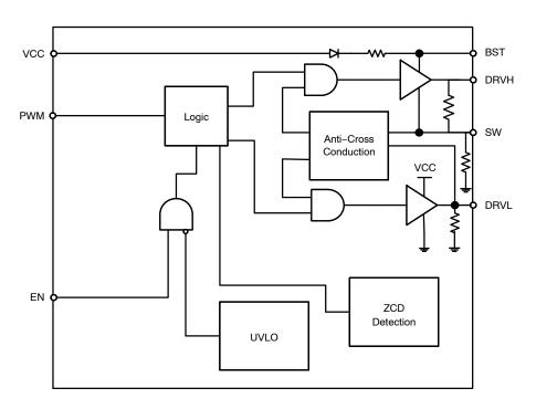
Figure 1. Block Diagram
