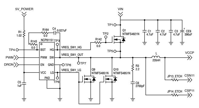
Figure 2. Application Circuit
