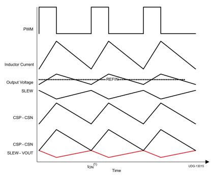
Figure 20. On-Time Waveforms <sup>(1)</sup>
