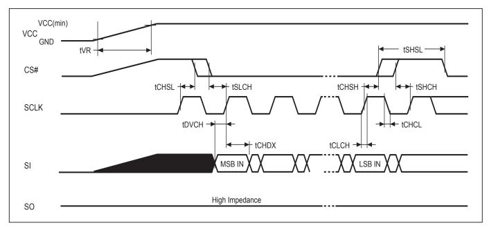
Figure A. AC Timing at Device Power-Up
