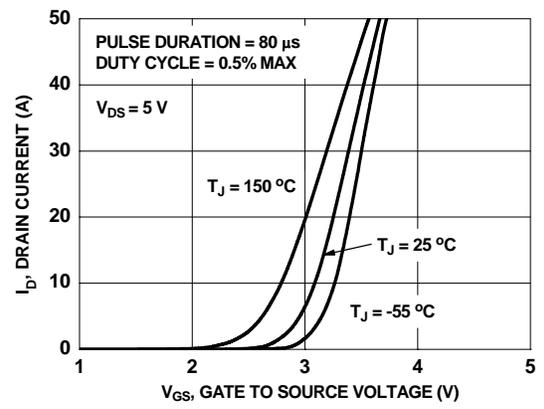
Figure 5. Transfer Characteristics
