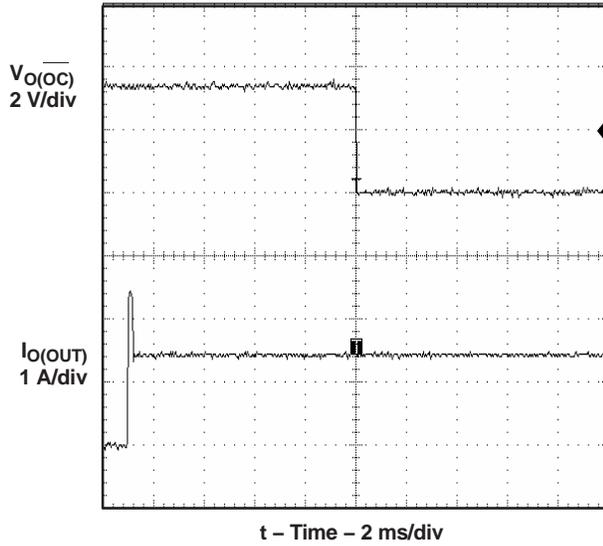
Figure 8. 2-Ω Load Connected to Enabled Device
