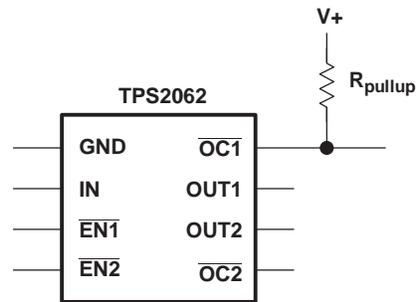
Figure 26. Typical Circuit for the  $\overline{\text{OC}}$  Pin
