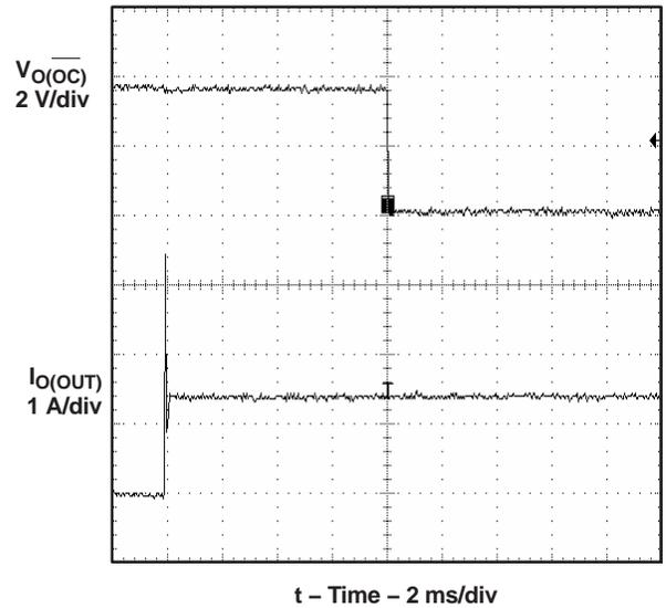
Figure 9. 1-Ω Load Connected to Enabled Device
